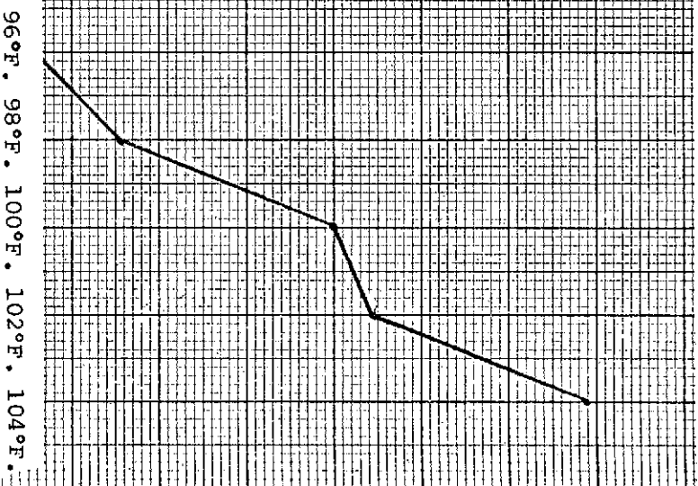
AFS SPEED VS. FIRST DEVELOPER TEMPERATURE
