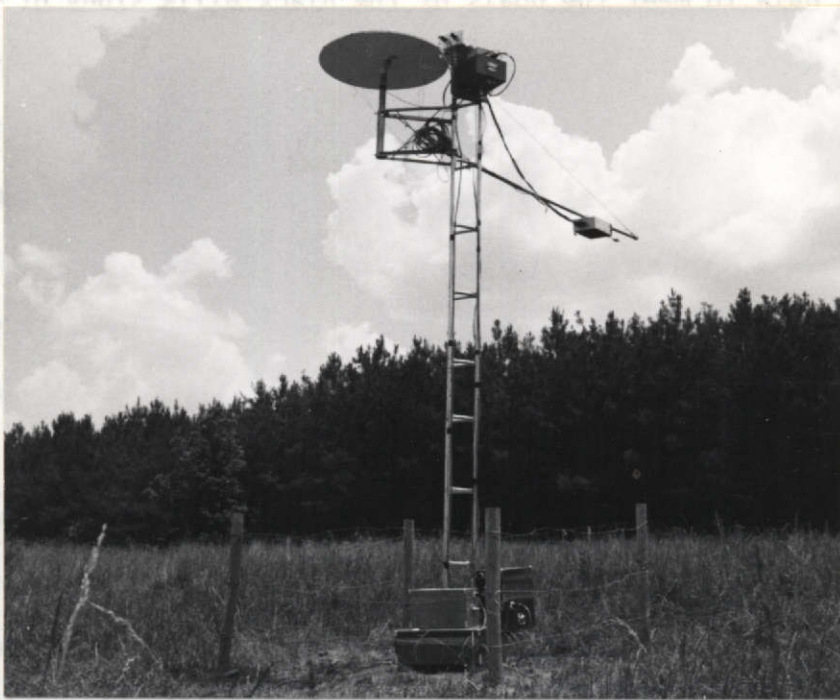
Figure 20. Modification of the data transmission network during the ERTS-1 experiment resulted in each subsite becoming an independent unit. Shown at the top of the tower are the incident-energy spectrometer, multiplexer, DCP, antenna, and light-activated switch. The reflected energy spectrometer is at the end of the 4-meter (13-foot) boom arm and the alkaline battery power packs are at the base of the tower.
