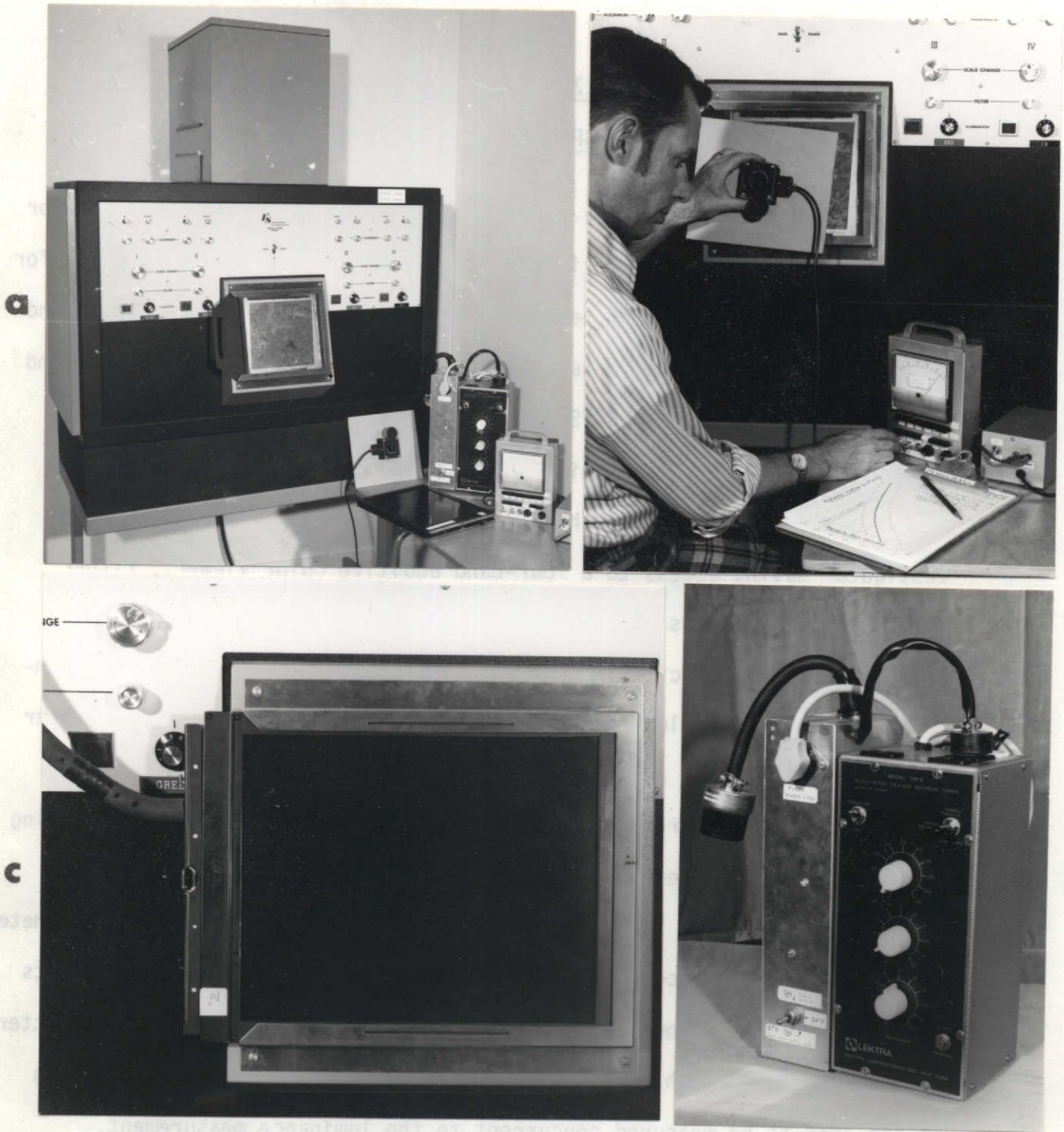
Figure 35. Equipment required to make color internegatives from ERTS 70 mm transparencies. (a) I 2 S additive color viewer with photometer and high-speed timer, (b) Forest Service-designed photometer being used to measure light intensity of each MSS band and of color composite, (c) 8- by 10-inch vacuum film holder--note vacuum hose on left, and (d) Lektra Decade Interval Timer (right) with heavy-duty relay and switching circuit box (left).
