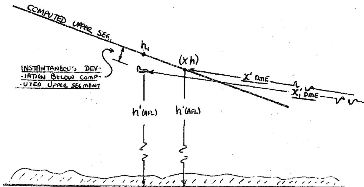
FIGURE 1 - UPPER SEGMENT DEVIATION - DME vs AFL
