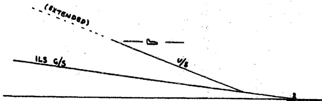
1. All system validity checks and navaid inputs proper. Aircraft has passed (or is physically above) upper segment. Pilot configures for two-segment approach (ILS tuned, 2-SEG switch to "ARM"; F/D and/or autopilot to respective auto mode.)
