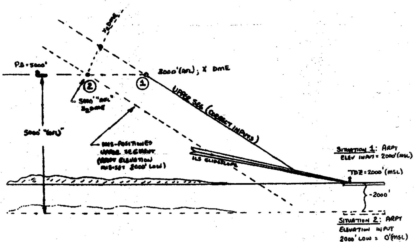
Situation 1: Aircraft is proceeding inbound at 5000' baro corrected pressure altitude for a two-segment approach to a runway with published TDZ of 2000' (MSL). The airport elevation
