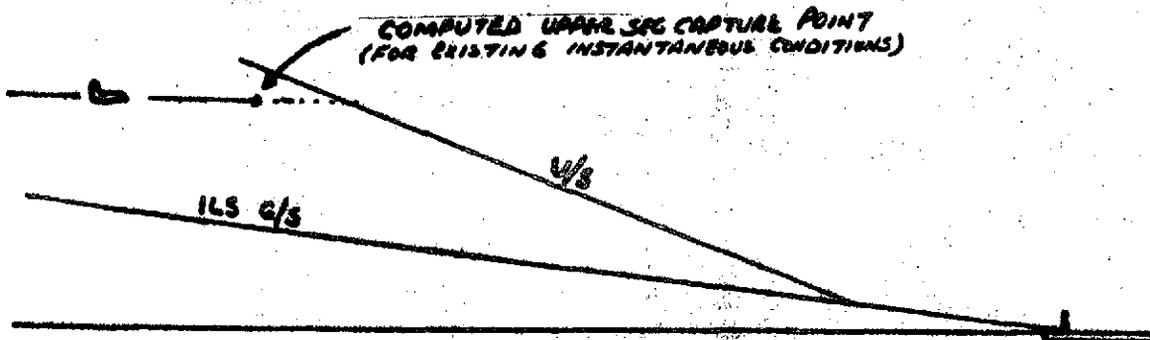
1. Two-segment switch in "ARM". NAV receiver tuned to ILS. Glideslope receiver section inoperative.
