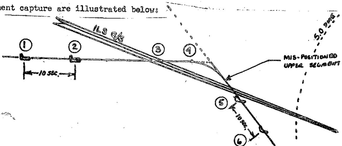
FIGURE 7 - BELOW-TO-ABOVE GLIDESLOPE PRIOR TO
