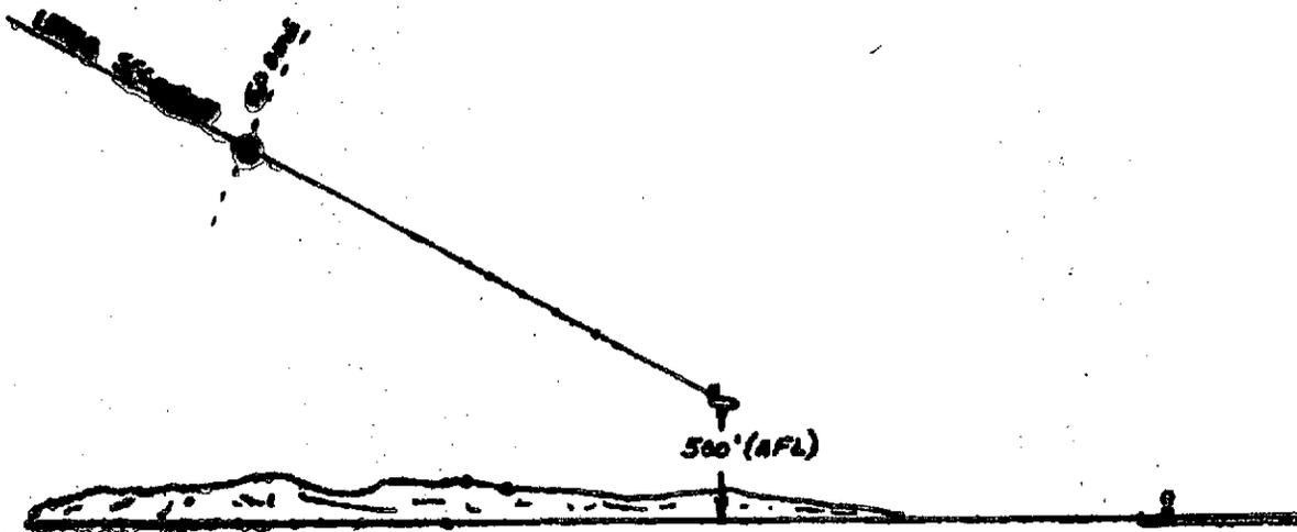
**Situation:** Aircraft is descending on upper segment. ILS glideslope has failed, or glideslope deviation protector ( **I** above) has not activated for some unknown reason.
