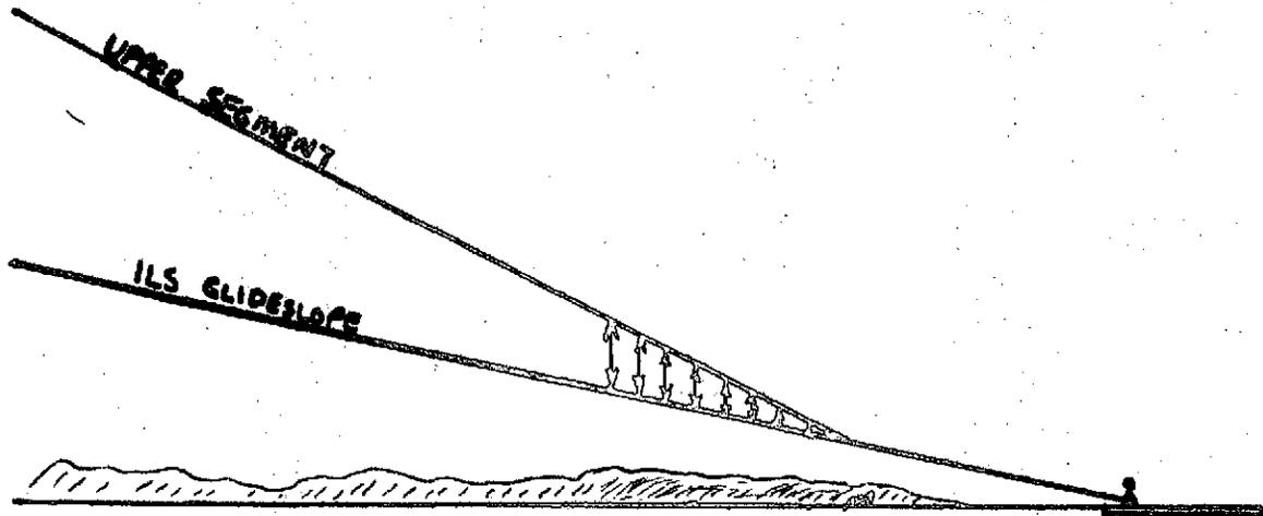
FIGURE 3 - SIMULATOR PROGRAM PROVISION FOR VARYING GLIDESLOPE CAPTURE POINT.
