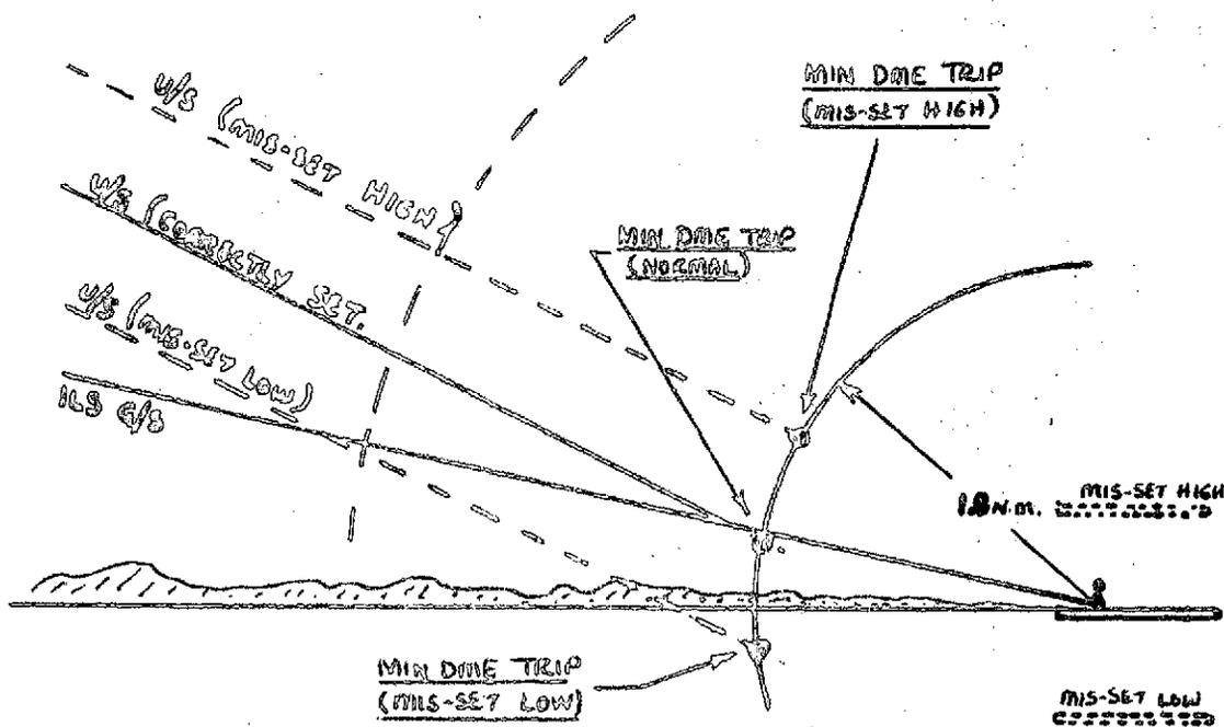
FIGURE 5 - MINIMUM DME TRIP - INCLUDING EFFECT OF MIS-SETTING AIRPORT ELEVATION HIGH OR LOW.
