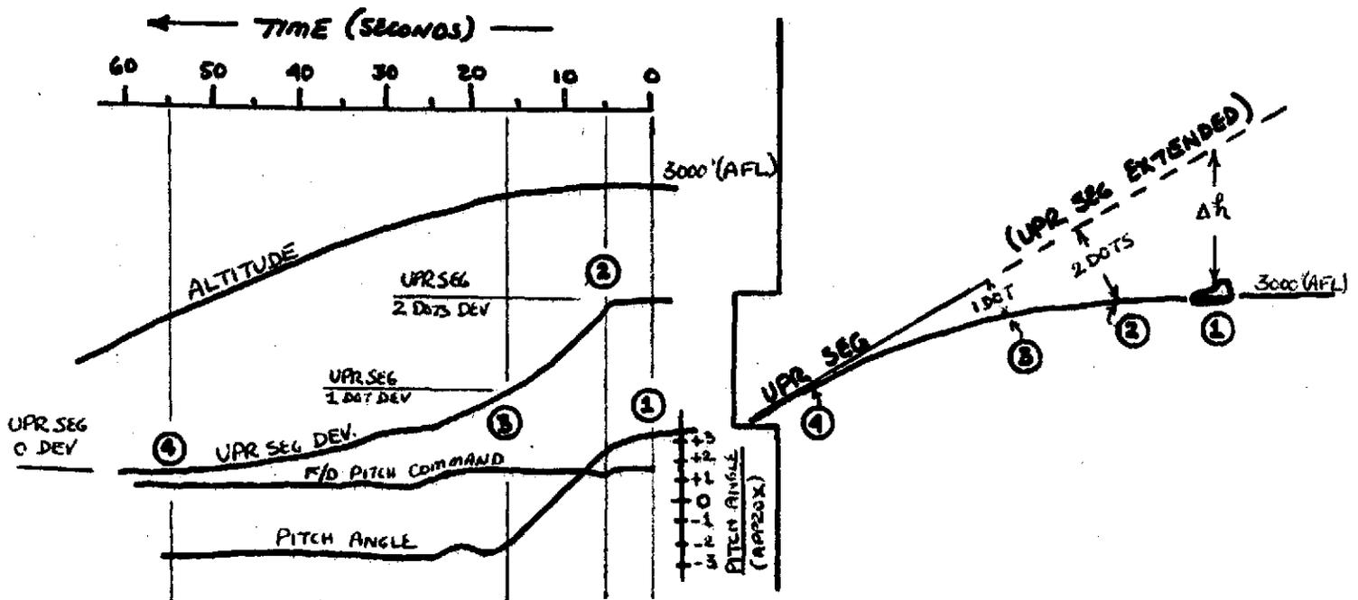
FIGURE 2 - UPPER TRANSITION OSCILLOGRAPH DATA RELATED TO AIRCRAFT POSITION IN PROFILE
