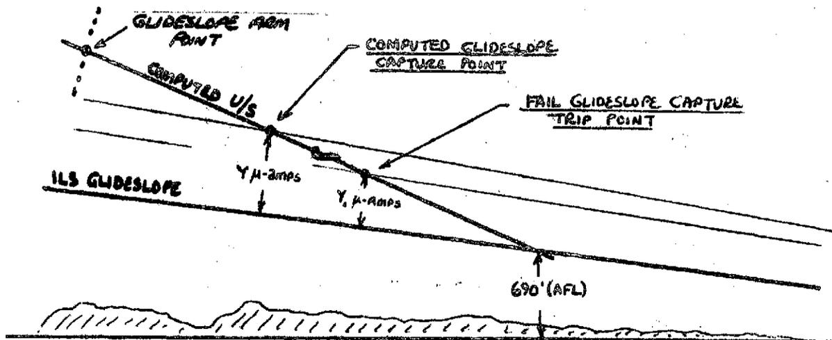
FIGURE 3 - GLIDESLOPE DEVIATION PROTECTOR - FAIL GLIDESLOPE CAPTURE
