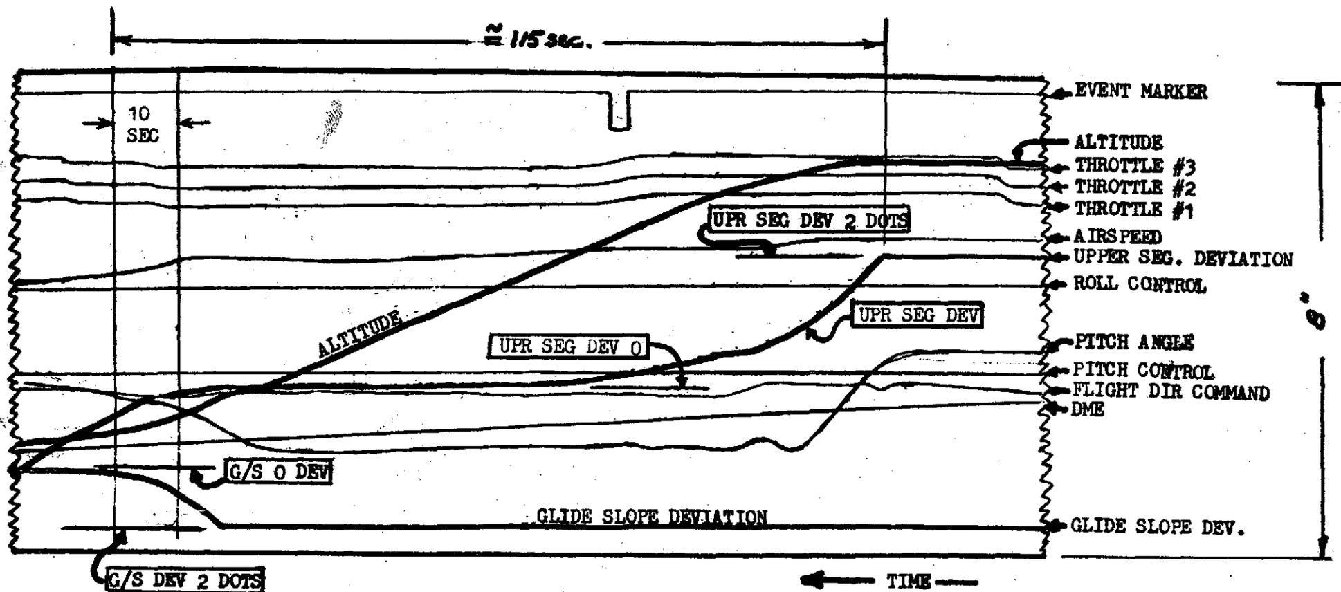
NOTE: The above is a copy of an actual data trace showing a 2-segment approach 6° Upper Segment 2.5° Glide Slope. Initial approach altitude 3030' MSL.
