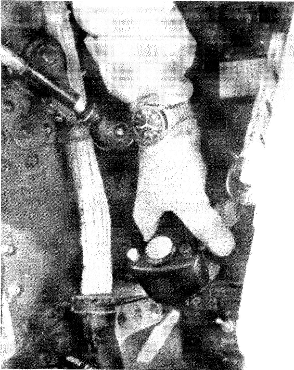
Figure 7. Force side stick in F-8 digital fly-by-wire airplane.
