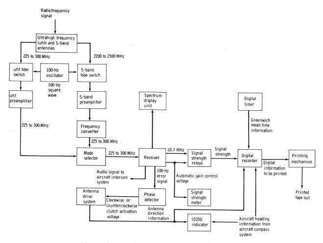
Figure 1. - Block diagram of the AN/ARD-17.
