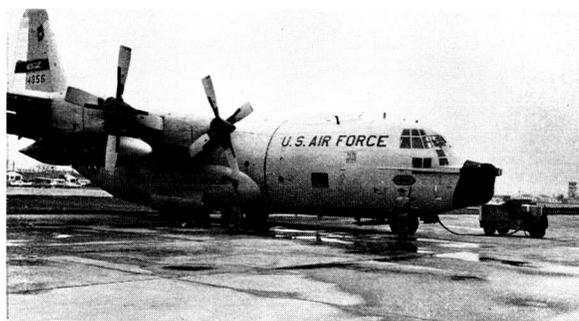
Figure 3. - A USAF HC-130 aircraft, showing AN/ARD-17 radome.
