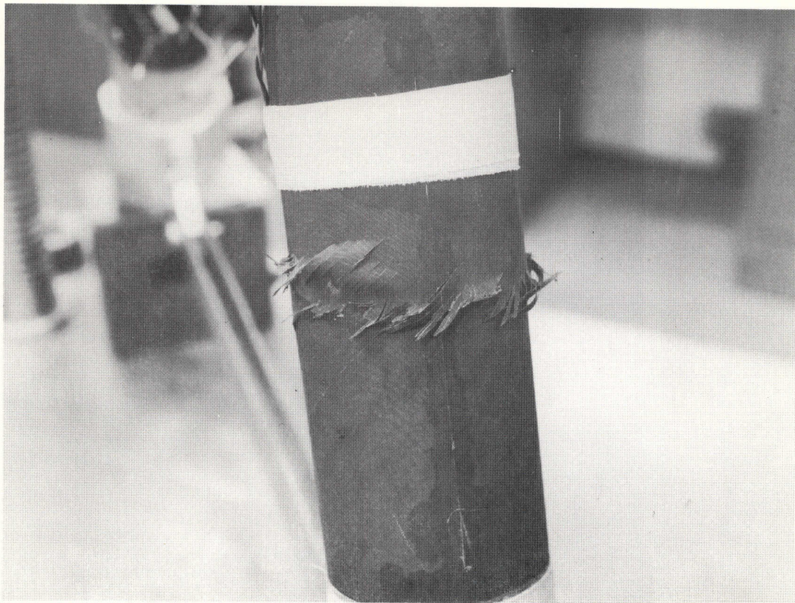
Figure 2-39 Component Failure-Close-Up of Far Side
