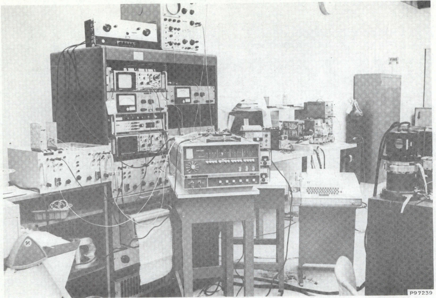
Figure 17. Test Set-up of Converters and Interface for Digital Compensation Loop System
