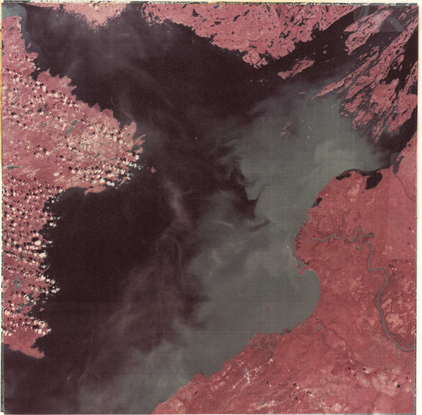
Figure 8.1. ERTS-1 image of the center of Great Slave Lake, District of MacKenzie, Canada, August 16, 1972, showing lake turbidity.
