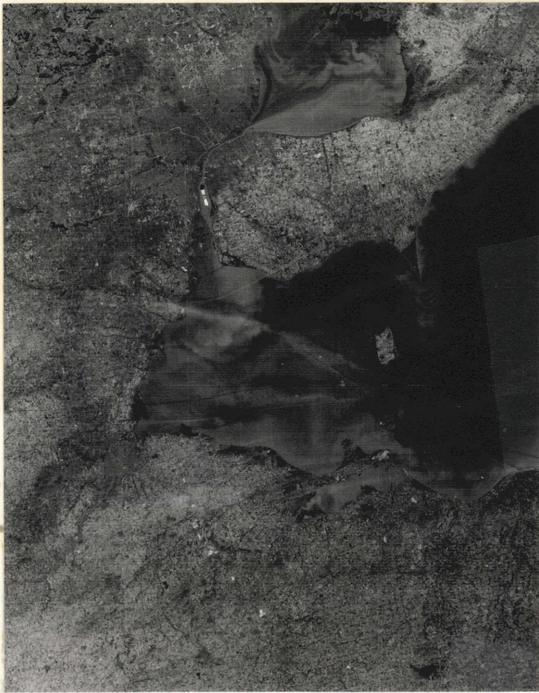
Figure 5.2. ERTS-1 MSS band 5 image of Lake St. Clair and western Lake Erie useful for Lagrangian current measurements using turbidity, April 14, 1973.
