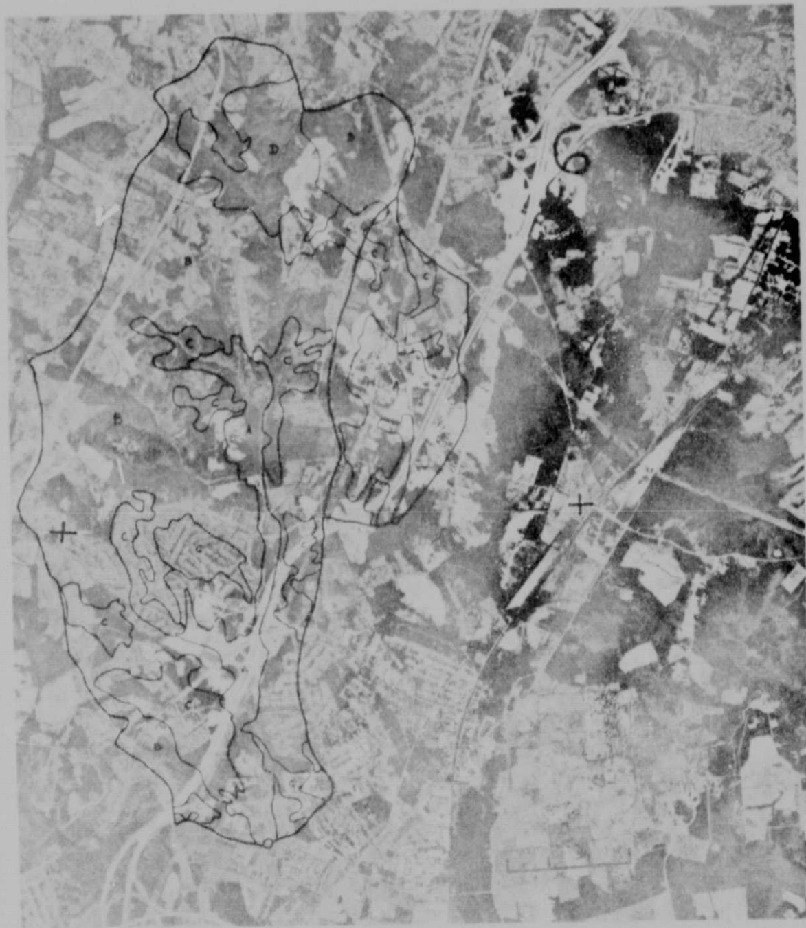
Figure 6. Slope map of Little Paint Branch and Sub-basin of Indian Creek, A = 0 to 2 percent, B = 2 to 5 percent, C = 5 to 15 percent, D = 15 to 25 percent. Approximate Scale 1: 56, 250.
