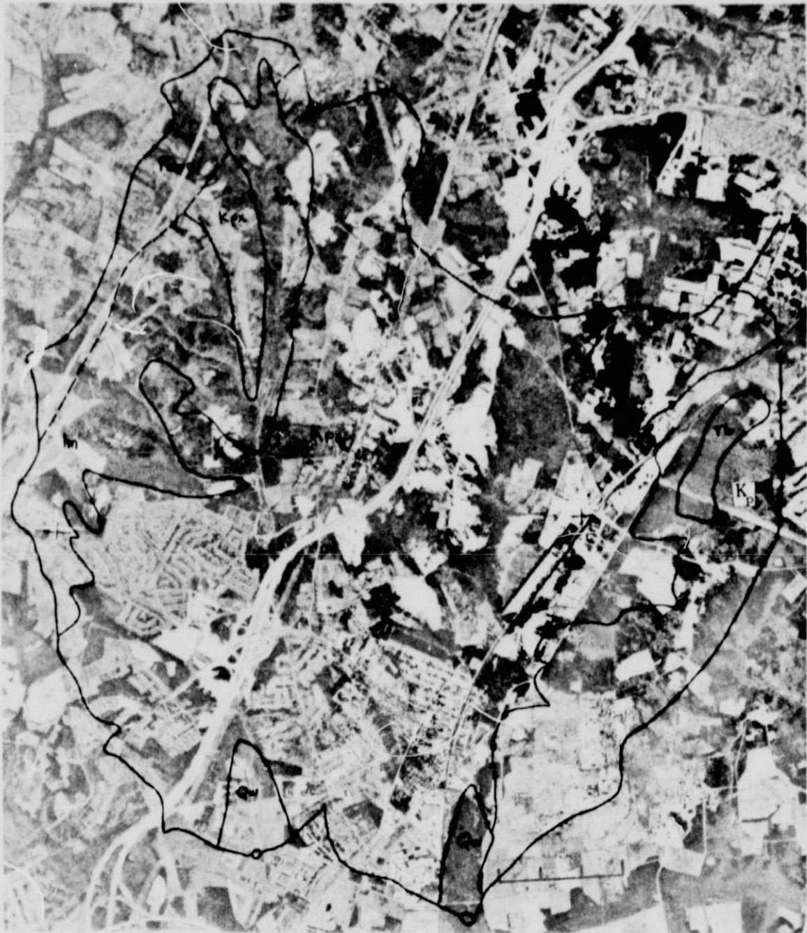
Figure 3. Geology map - see Table 16 for description of Geology. Note extent of Patuxent Formation (KPX) which is a major aquifer. Approximate Scale 1: 56, 250.
