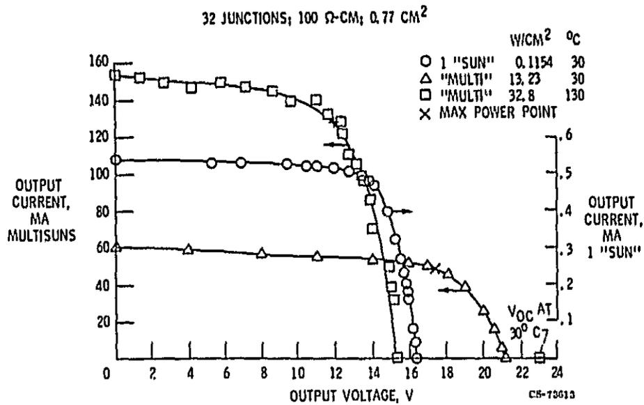
Figure 7. - I-V characteristics of HI cells at various intensities.
