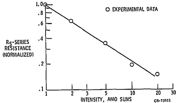
Figure 6. - HI cell series resistance normalized vs. intensity.
