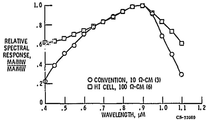
Figure 4. - Relative spectral responses of conventional and HI cells.
