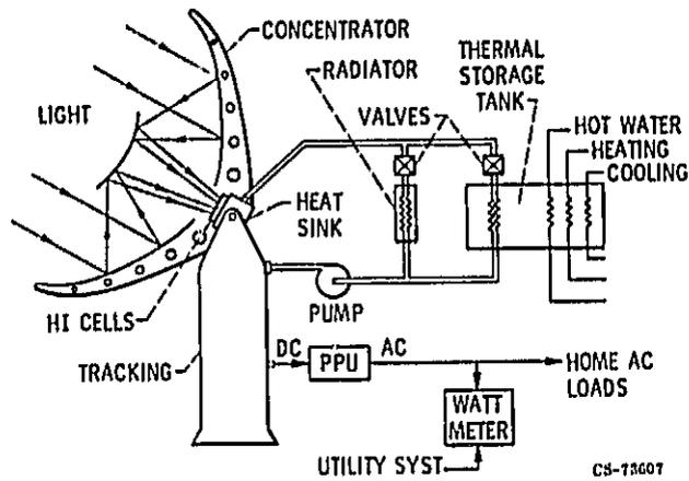
Figure 9. - High Intensity solar system.
