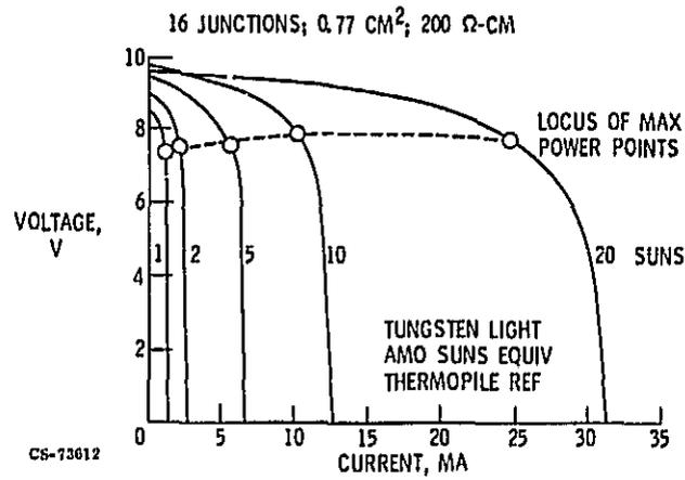
Figure 5. - HI cell I-V characteristics at various intensities.
