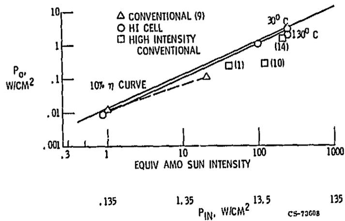
Figure 8. - Power output density at various intensities.
