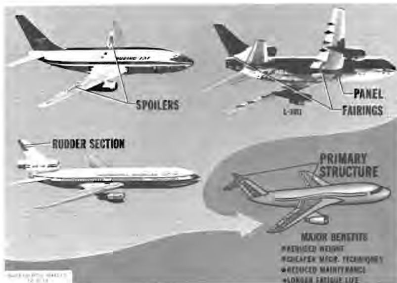
Figure 4. - Secondary structural components made of composite materials in operational use today on aircraft. (Later, composites will comprise primary structures yielding even greater benefits.)
