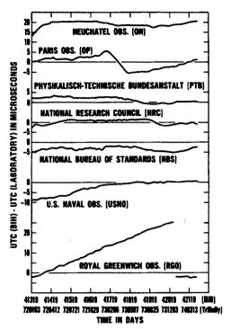
Fig. 4—Coordinated Universal Time (UTC) Scale of Individual Laboratory Relative to UTC (BIH)
