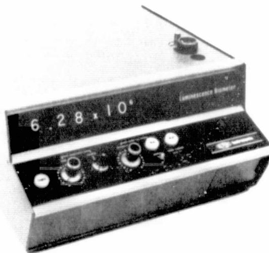
Biometer detects light response from firefly reaction.
