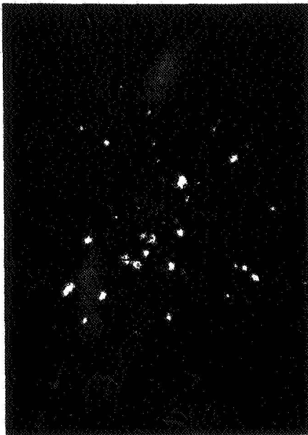
Figure 4. X-ray test photographs of a rare-earth phosphor/multi-stage intensifier system (Single x-ray photons at 60 keV and 122 keV are visible. Intensifier input diameter is 25 mm. X-ray spot size is \sim 0.5 mm. The centroid of each spot can be determined to less than 0.2 mm.)
