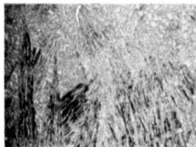
(b) MICROSTRUCTURE OF THE BLED-OUT REGION ("A") SHOWING FULL EUTECTIC STRUCTURE. LIGHT PHASE Ni-Cr SOLID SOLUTION AND DARK PHASE INTERMETALLIC.
