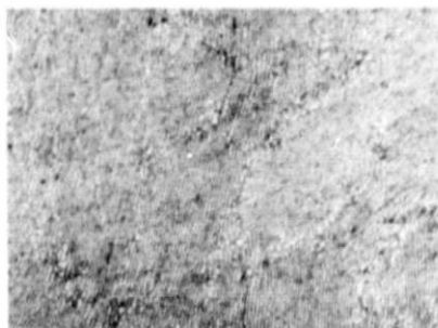
Figure 6. - Microstructure of directionally solidified Ni-19.2 Cr-14.8 Zr eutectic alloy, R = 1.0 cm/hr.
