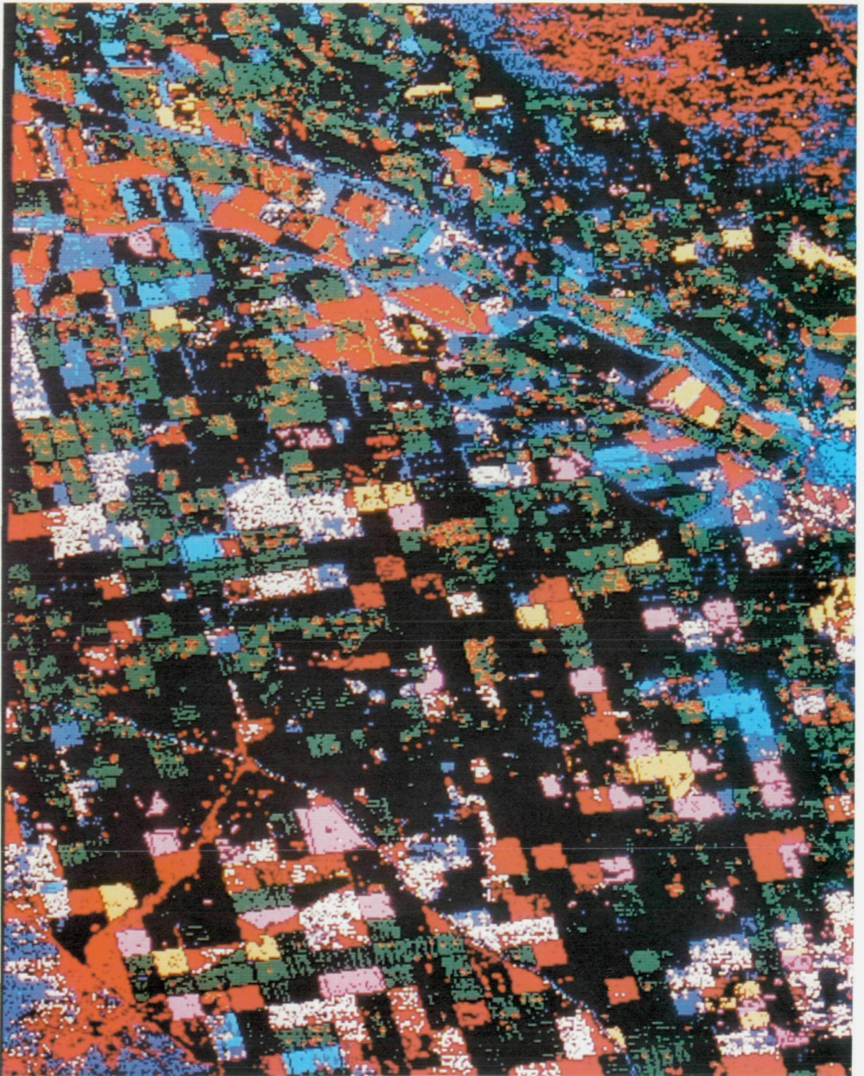
Figure 21.—Color-enhanced image showing results of supervised classification (yellow—barley stubble; brown—turned barley stubble; white—fallow; light blue—burned barley stubble; dark blue—water and flooded fields; pink—safflower; red—rice; green—mature crops; black—all others).
