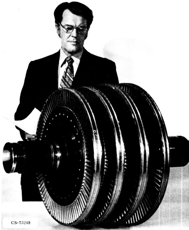
Figure IX-60. - Fan turbine rotor.
