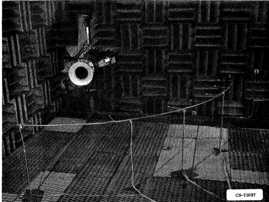
Figure I-23. - Model fan in Langley anechoic chamber.
