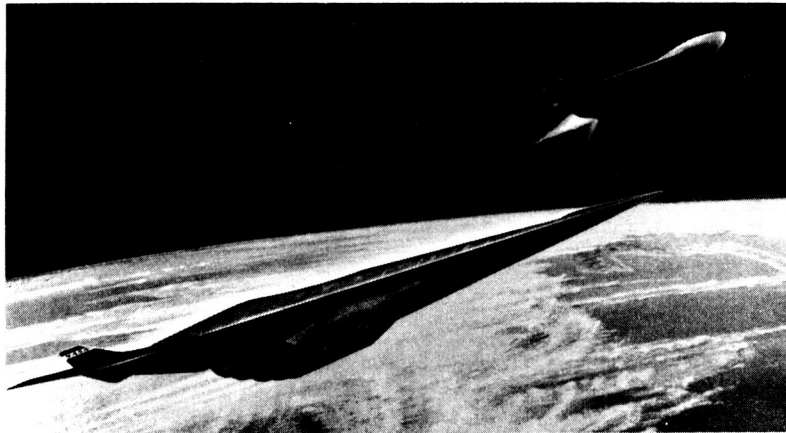
Figure XV-1. - Airbreathing launch vehicle designed for hypersonic speeds.
