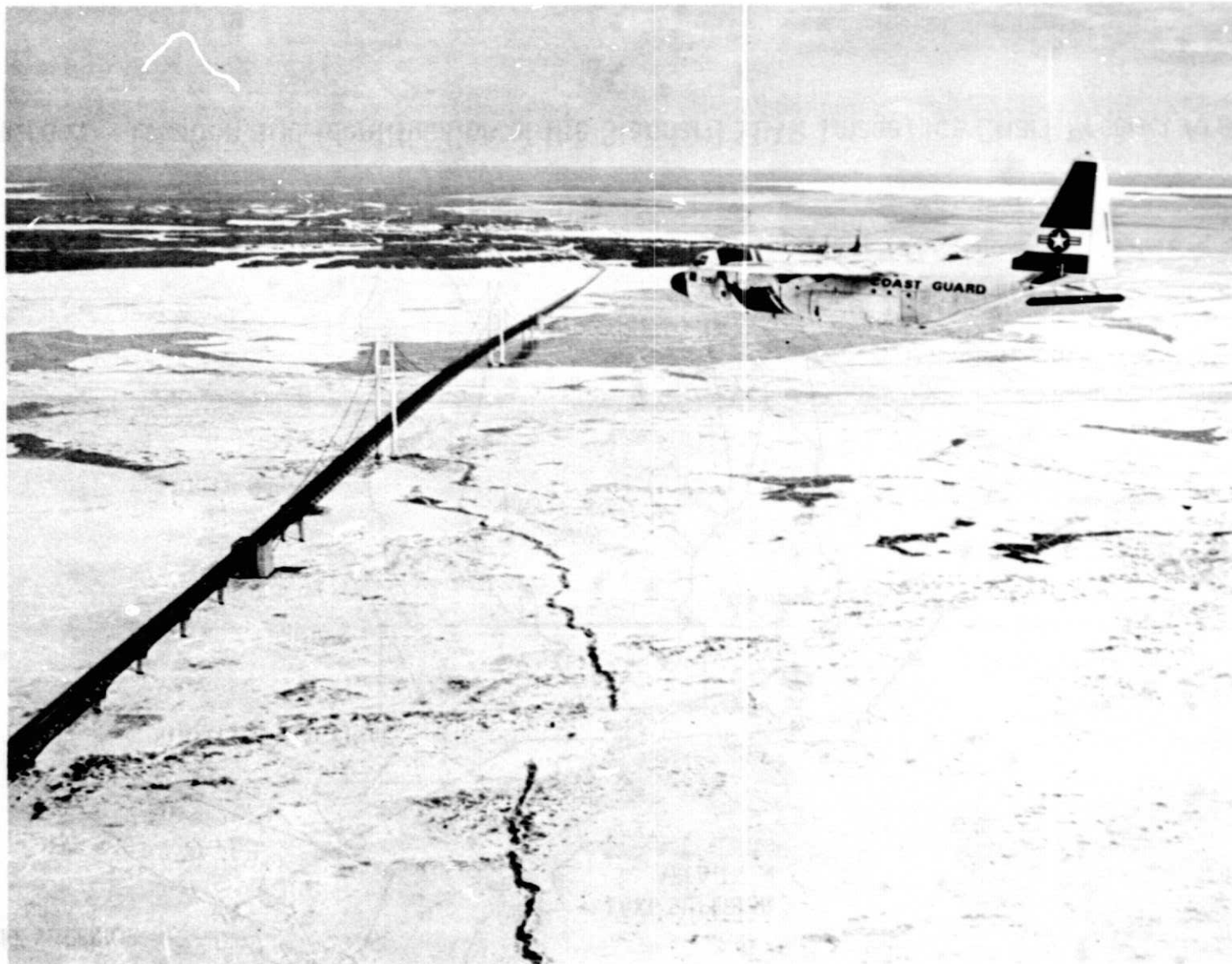
Figure 3. - Photograph of the U. S. Coast Guard C-130 B SLAR aircraft used in the 1974-75 Winter Ice Program. The ice cover around the Mackinac Bridge is shown in the background.
