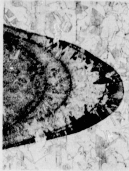
Figure 10. Ground-base and Skylab EB melts in 304 stainless steel (photographically reduced 18 percent for publication).
