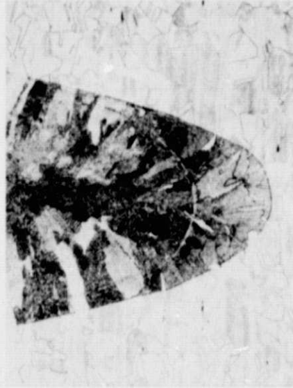
Figure 10. Ground-base and Skylab EB melts in 304 stainless steel (photographically reduced 18 percent for publication).
