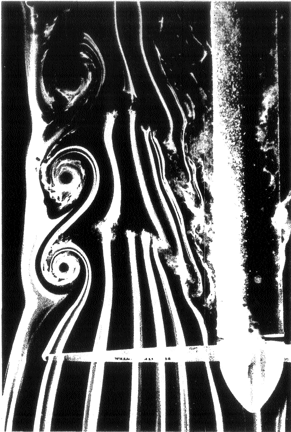
Figure 9. Flow Visualization of a Two-Bladed Propeller (Professor F.N.M. Brown's Propeller Smoke Picture - 1950)
