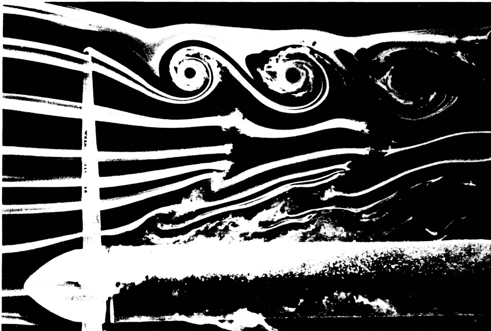
Figure 9. Flow Visualization of a Two-Bladed Propeller (Professor F.N.M. Brown's Propeller Smoke Picture - 1950)
