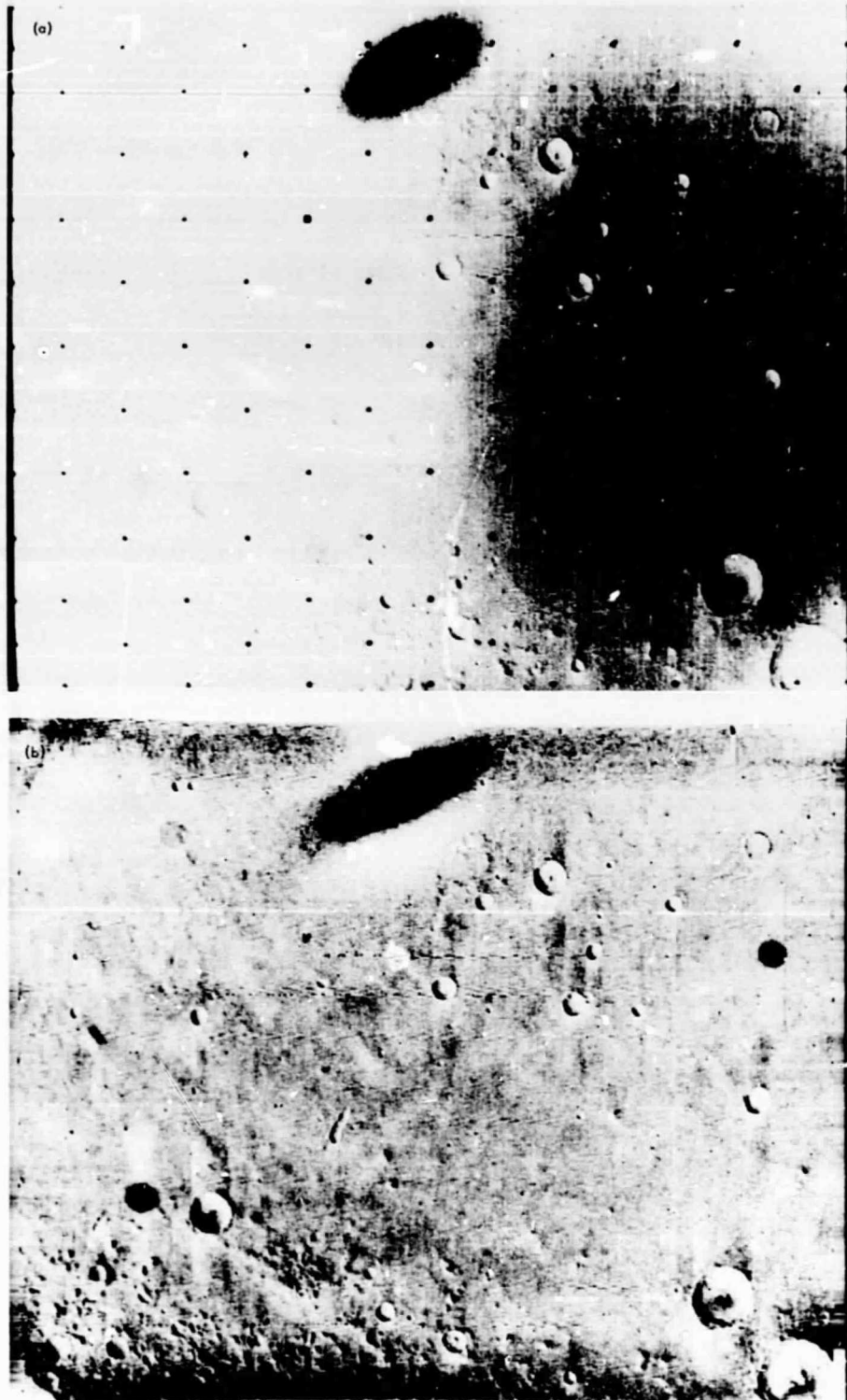
Fig. 3. RDR versions of the same Mariner 9 pictures shown in figures 1 and 2. The albedo version (a) has been given a linear stretch to preserve relative scene brightness across the image. The filtered version (b) has been processed to emphasize topographic detail. (IPL Roll Nos. 7350 and 1631.)
