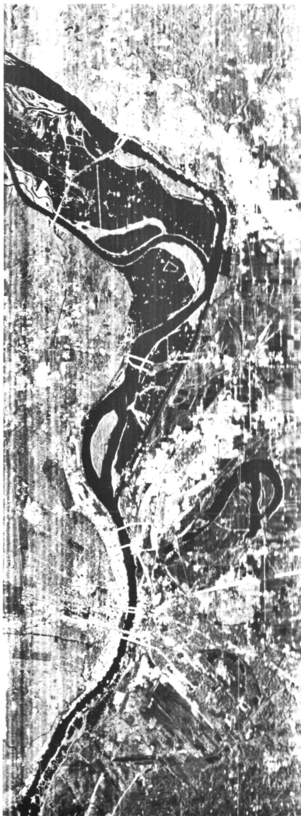
FIGURE 2-12.—Radar imagery of the May 1973 Missouri River flood. Water appears as black, which indicates areas of no signal return, because its surface is smooth to a wavelength of approximately 3 cm.
