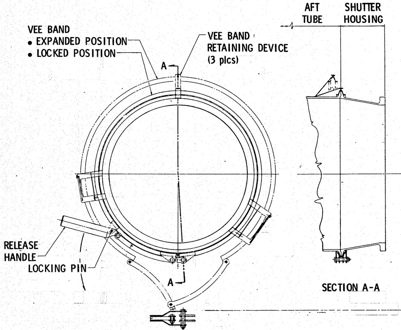
Figure 4-7. Shutter Housing/Aft Tube Interface Clamp
