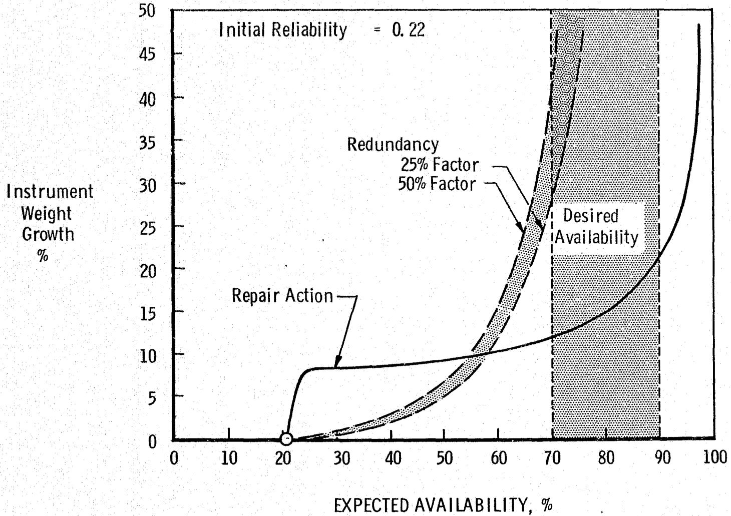
Figure 7-12. Redundancy versus Repair for S-056 (Initial Rel. = 0.22)
