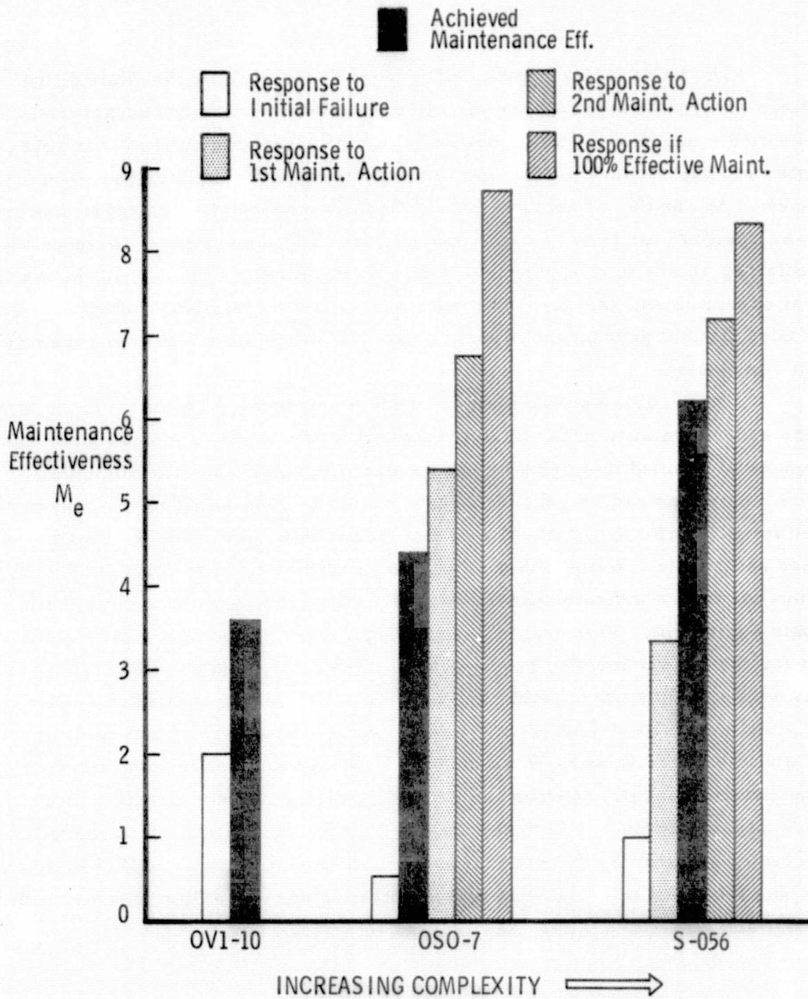
Figure 5-5. Maintenance Effectiveness for Three Types of X-ray Instruments
