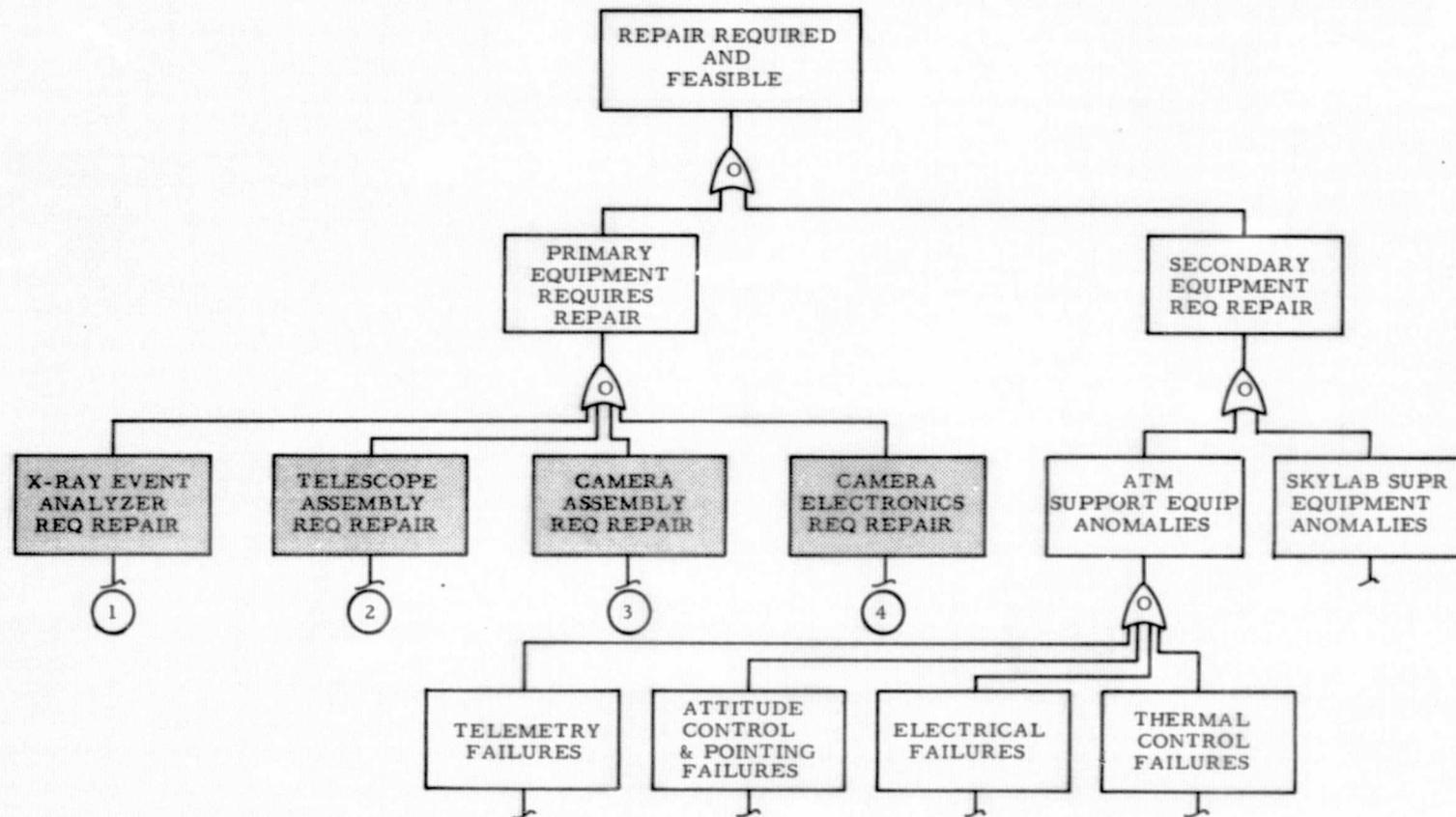
Figure 7-3. S-056 Second Level Fault Tree
