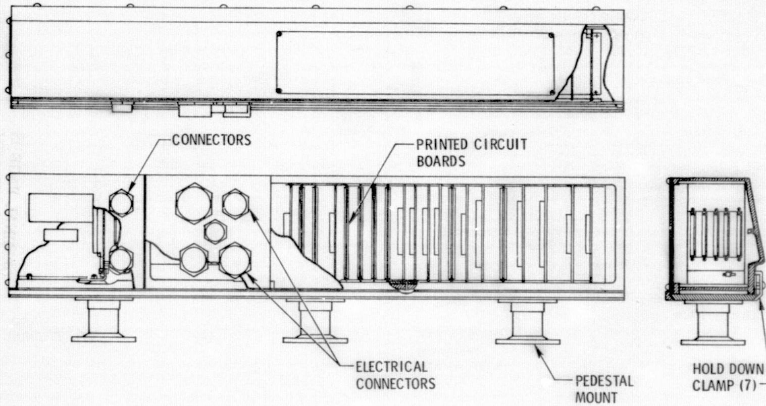
Figure 4-9. S-056 Camera Electronics Assembly
