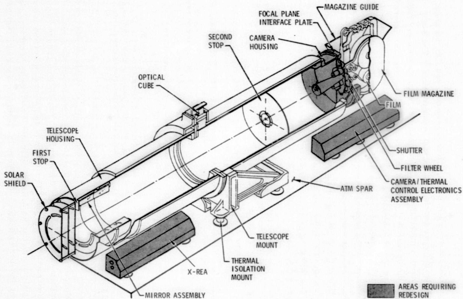
Figure 4-6. S-056 X-Ray Telescope Candidate Redesign Areas
