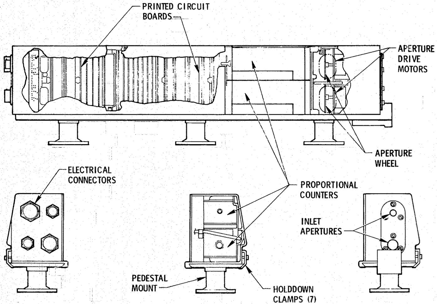
Figure 4-10. X-Ray Event Analyzer Assembly
