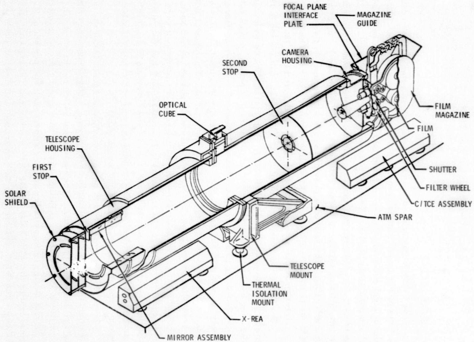
Figure 4-1. S056 X-Ray Telescope Configuration
