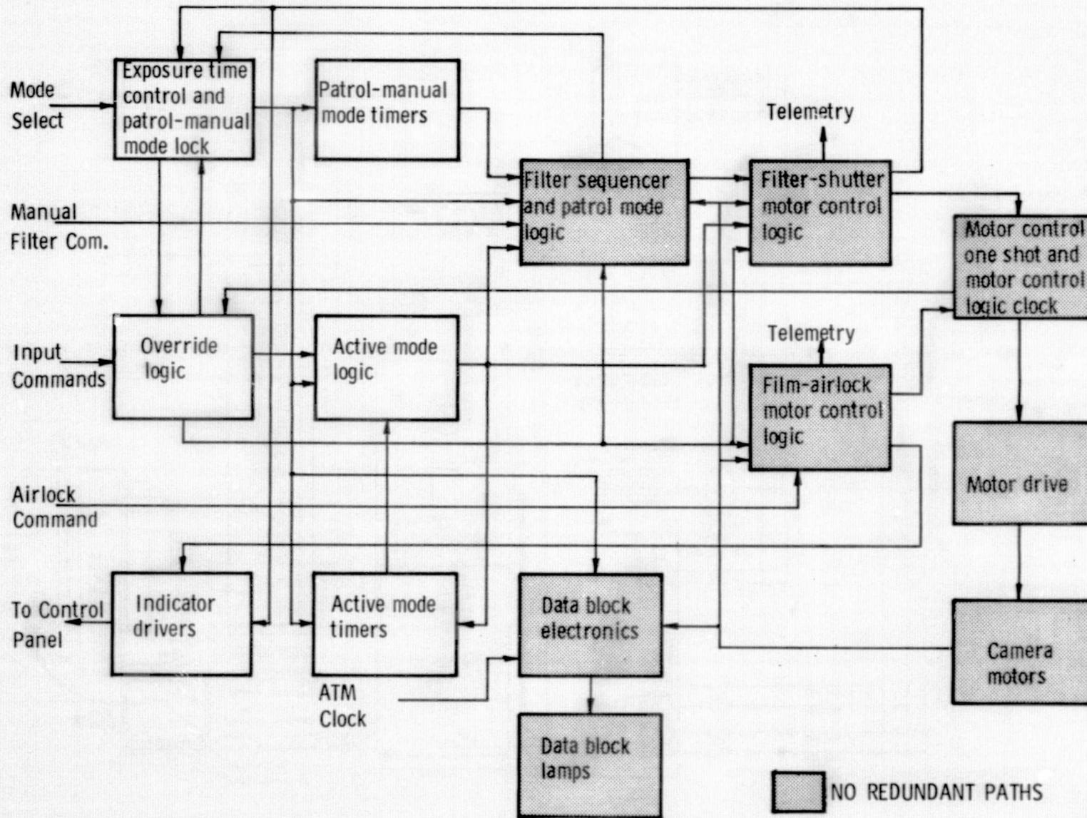
Figure 4-4. Functional Block Diagram of S-056 Camera Electronics
