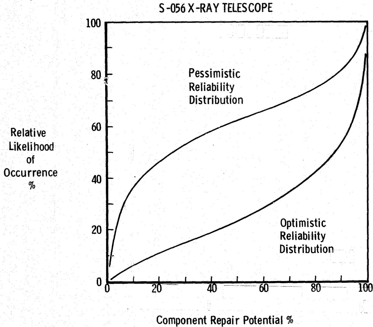
Figure 7-8. Alternate Component Repair Characteristics
