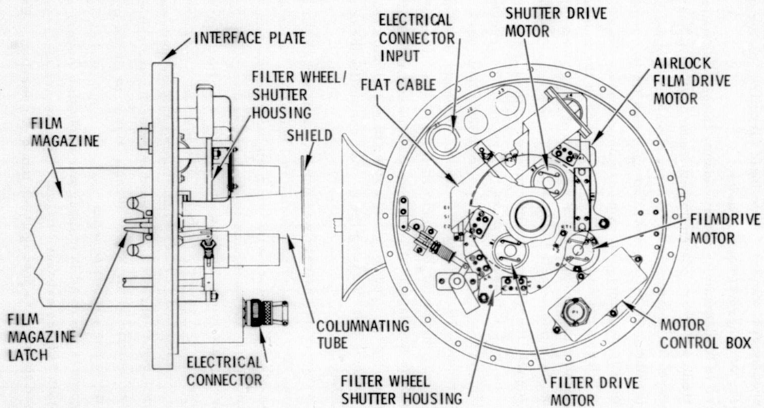
Figure 4-3. S-056 X-Ray Telescope Interface Plate/Shutter Assembly
