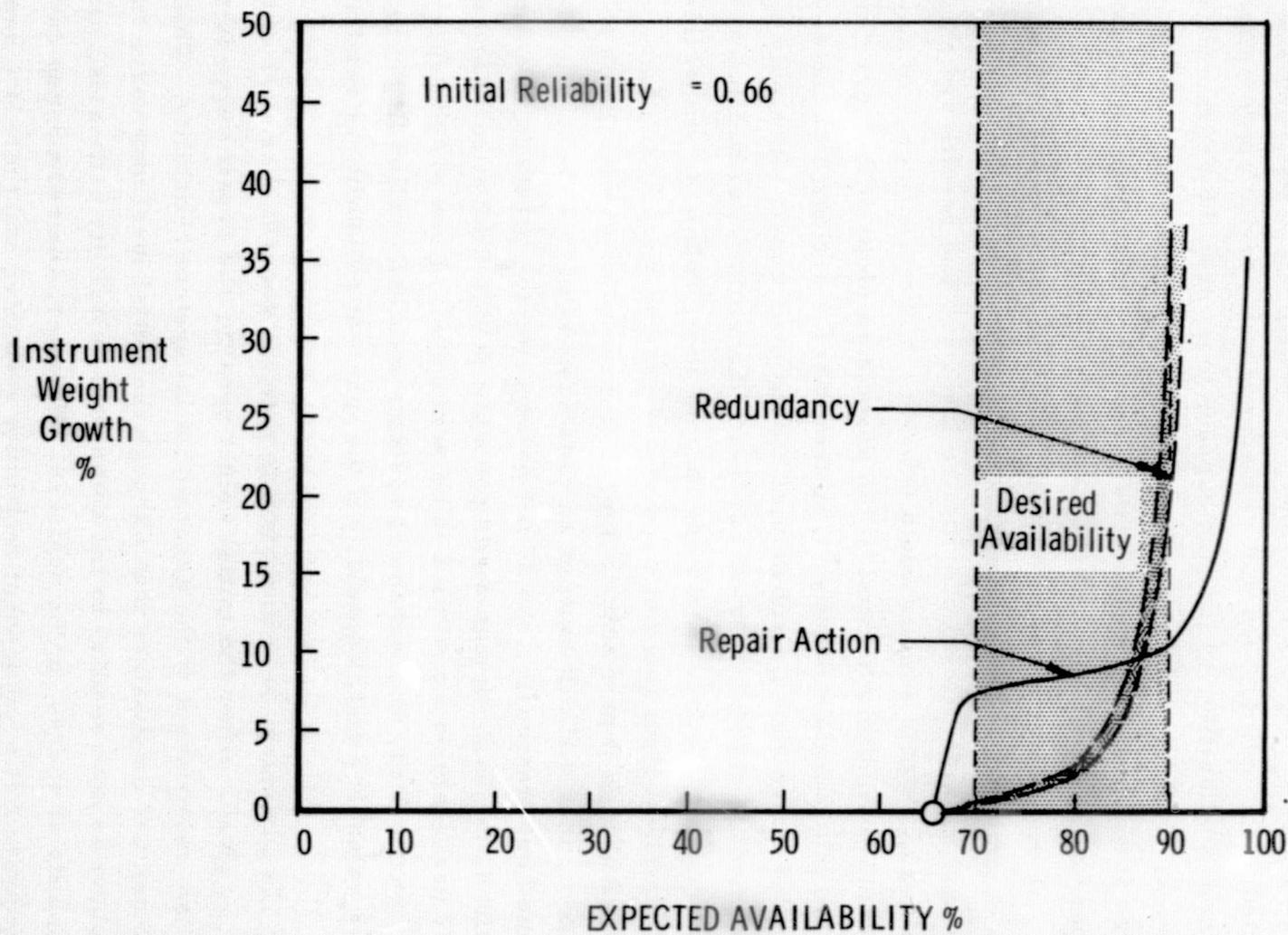
Figure 7-13. Redundancy versus Repair for S-056 (Initial Rel. = 0.66)
