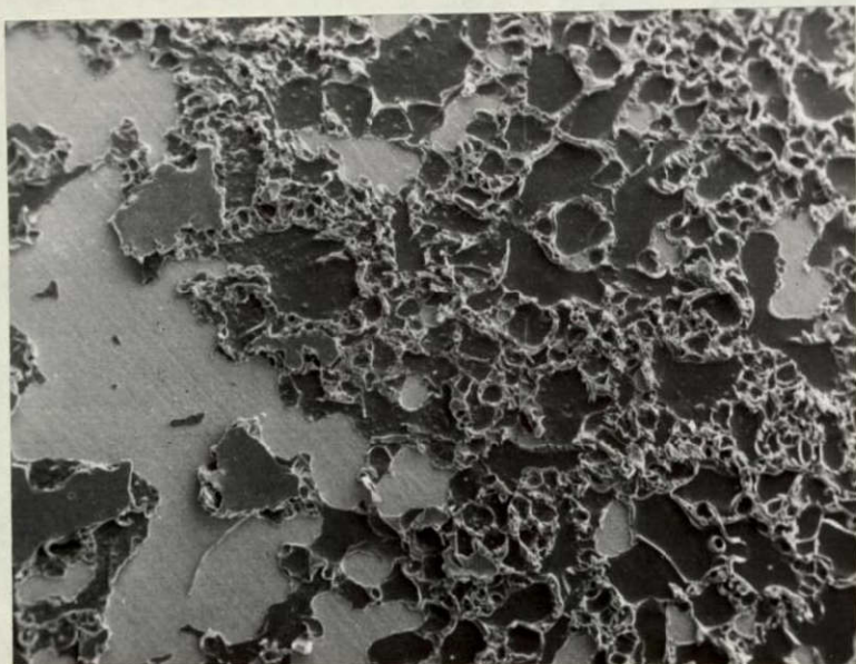
FIGURE 8. Two magnifications of the opposite mating fracture surfaces of sample #721D4 that gave 760 psi shear strength at 270°C after aging for 30 days at 295°C. Extensive interfacial failure, and small amount of plastic deformation and cleavage cracks.
