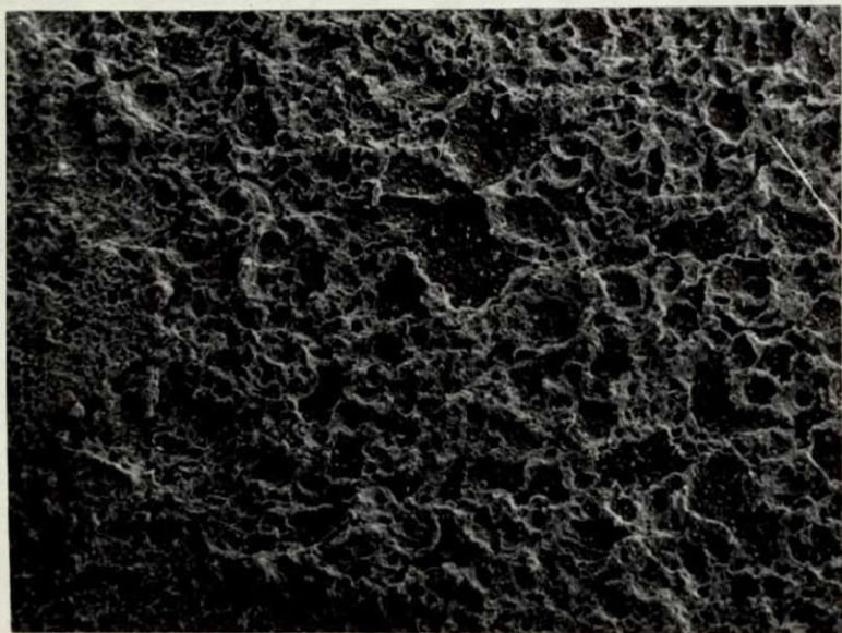
FIGURE 20. Two magnifications of sample #546D3 and #546D4, both with 50% Al, tested at 25° and 250°C, respectively. Shear strength dropped from 3775 psi to 1210 psi. "Melting" caused by high temperature and stress is visible in the lower right.
