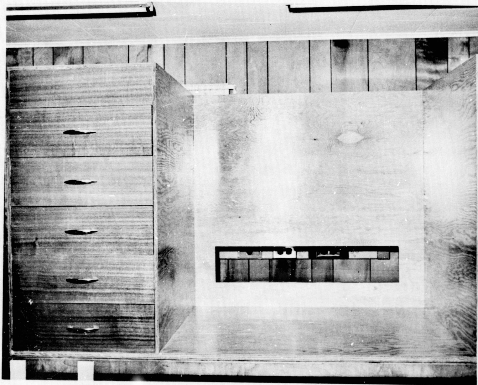
Figure 22.- Simulated Spacelab workbench; surface area = 0.57 \text{ m}^2 , storage volume = 0.15 \text{ m}^3 .
