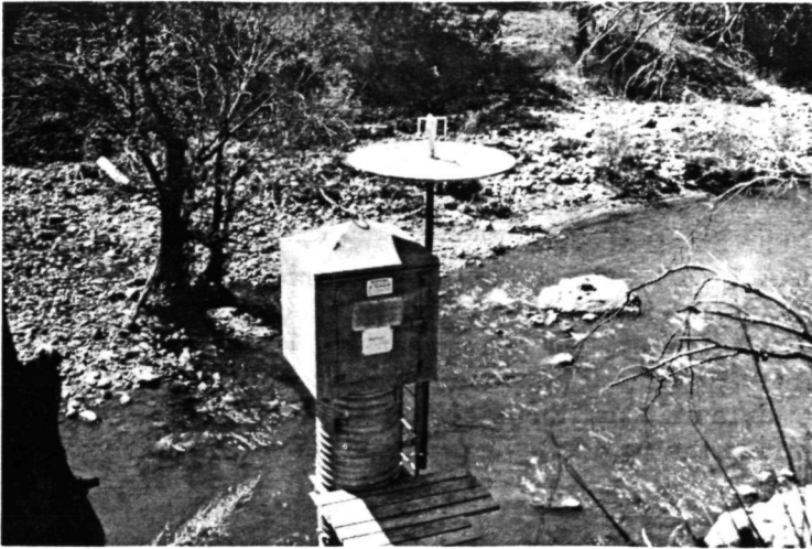
Fig. 7-White River streamflow gage near Ft. Apache, Arizona equipped with LANDSAT Data Collection Platform
