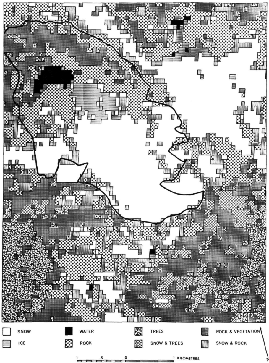
Fig. 6--Map of South Cascade Glacier area produced by computer recognition techniques. Black line is explained on Figure 7.
