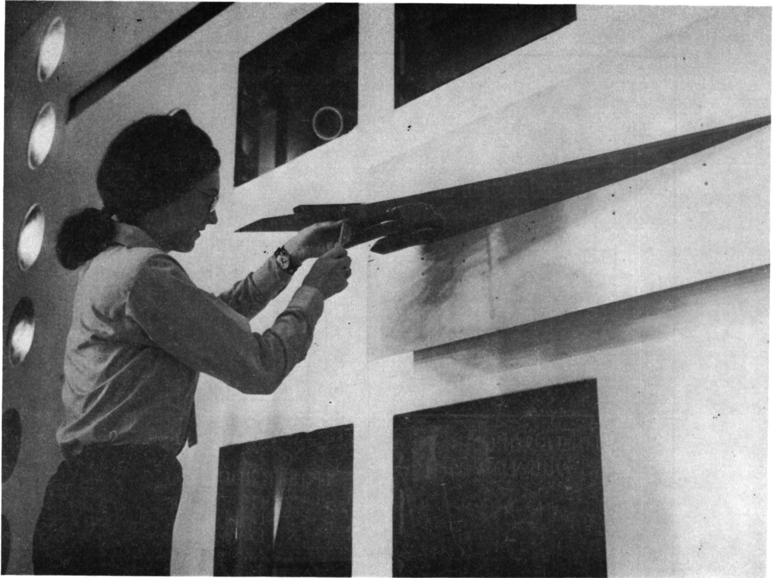
Figure 12.- Photograph of arrow-wing model mounted in wind tunnel.
