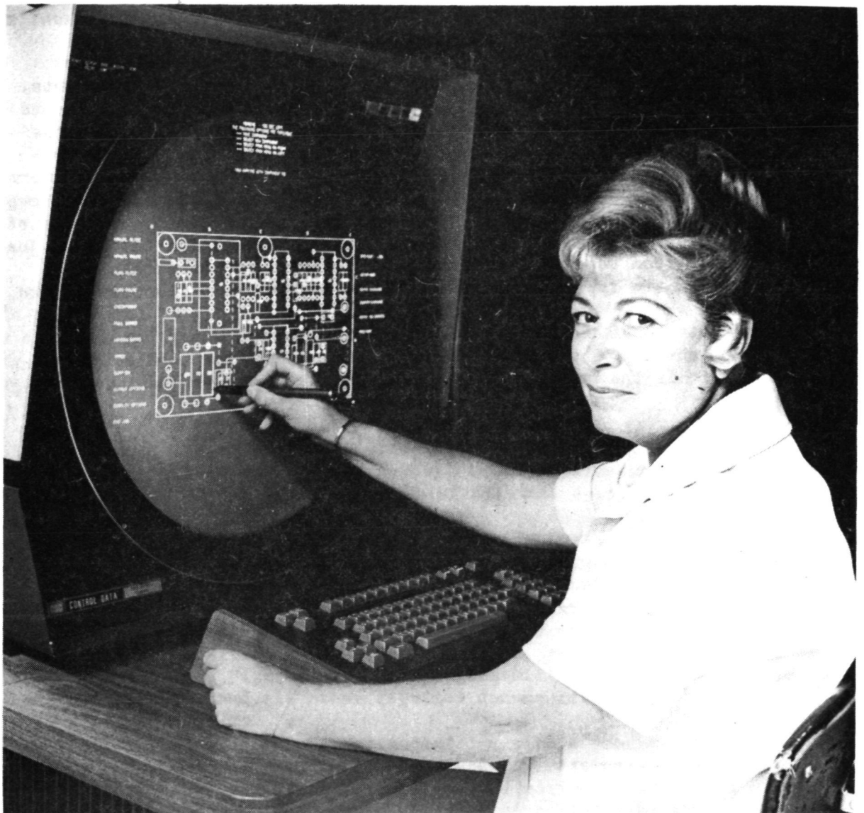
Figure 1. - Design engineer seated at the graphics terminal. The display screen, keyboard and light pen are the interactive elements of the system.
