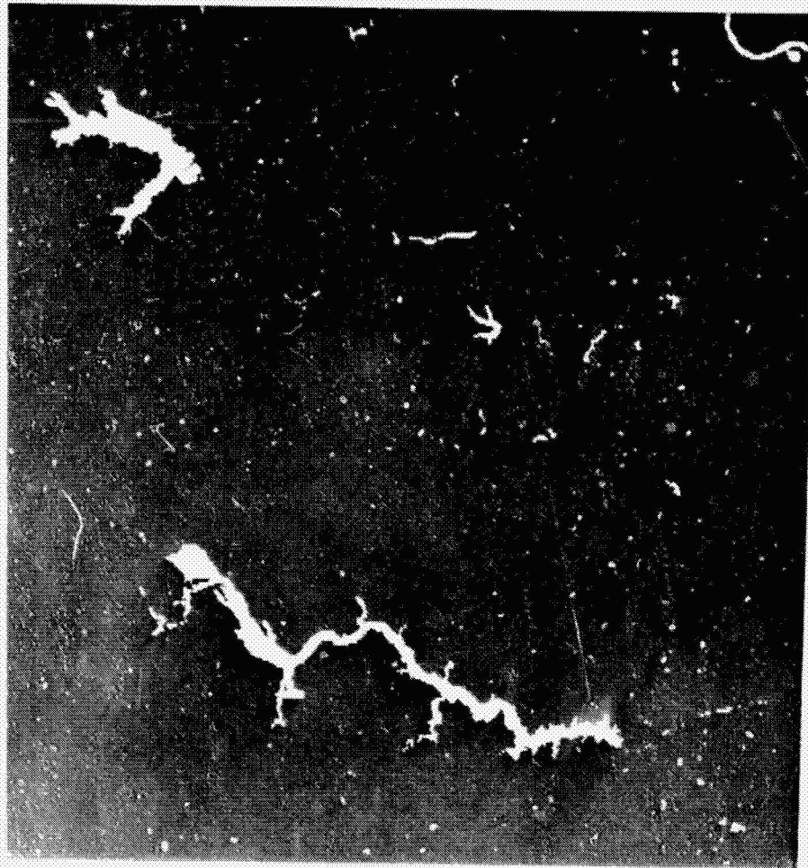
Figure 8.- Water inventory map of a 30 Km by 30 Km region SW of Richmond derived from a LANDSAT image by identifying all pixels which contained more than approximately 60% water.
