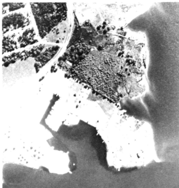
AQUATIC PLANT MONITORING - Entrance to Beacon Bay Marina. Cloudy patches offshore are areas of hydrilla infestation. (Enlargement of color infrared transparency).
