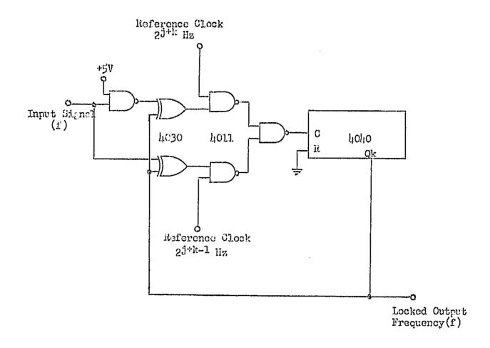
Figure 1. Binary Phase Locked Loop.
