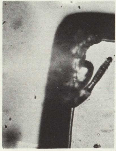
b) DIODE 5,3 CHIPPED DIODE (700X)
