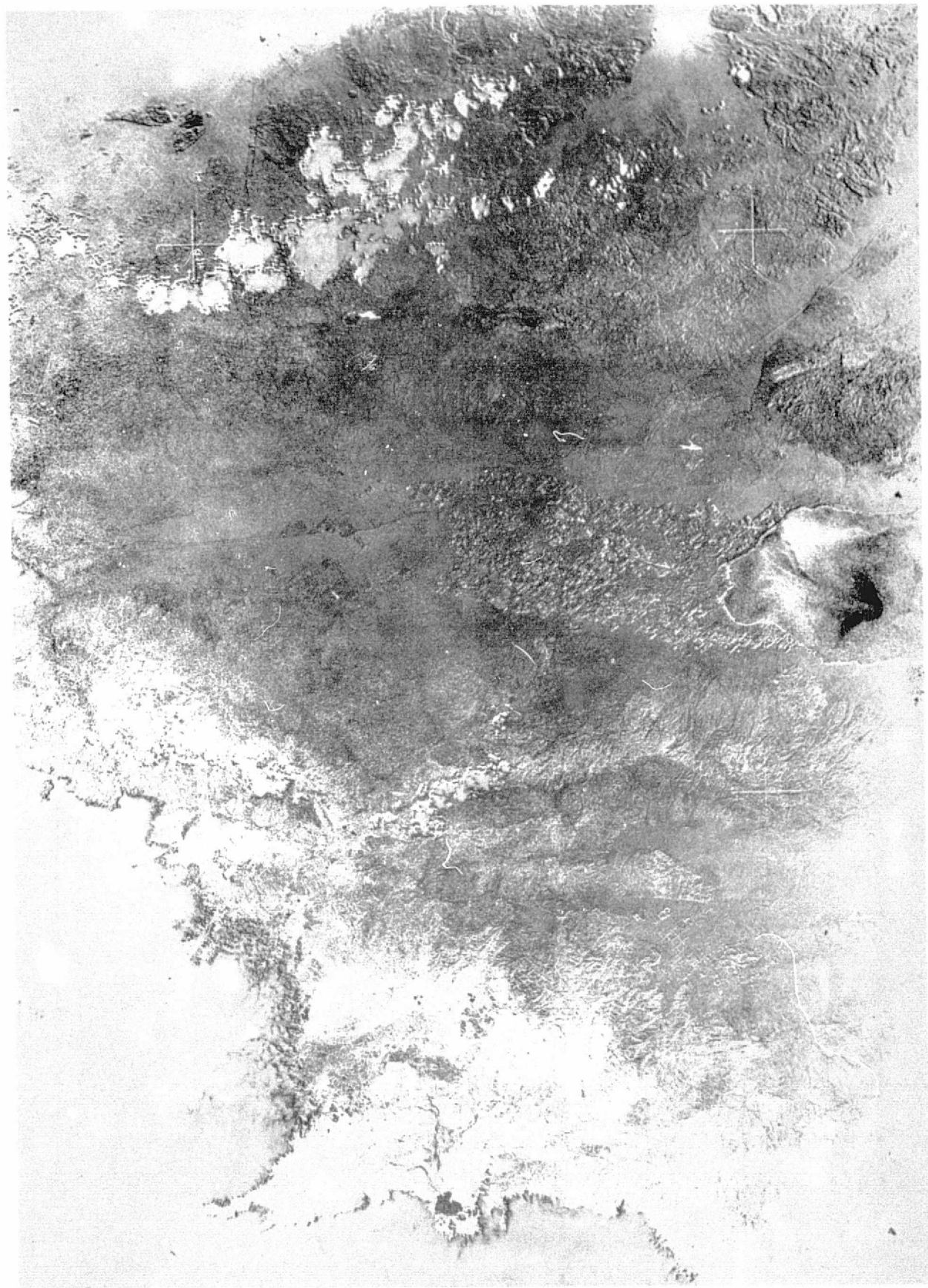
Fig. 13 - North end of Salton Sea and adjacent areas, southern California. Subtraction image prepared from Skylab 2, 190A camera images of bandwidths .5 to .6 \mu\text{m} and .6 to .7 \mu\text{m} , Pass 2, Track 63, Roll 5, Frame 114. See Fig. 11 for features identified.
