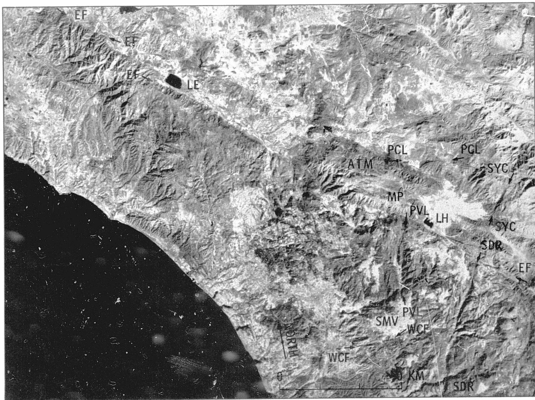
Fig. 5 - Major faults and linears, north central Peninsular Ranges, southwestern California. Portion of Landsat image 1125-17563. Abbreviations: ATM: Agua Tibia Mountains; EF: Elsinore fault; LE: Lake Elsinore; LH: Lake Henshaw; MP: Mount Palomar; PCL: Previtt Canyon linear; PVL: Pamo Valley linear; SDR: San Diego River fault zone; SMV: Santa Maria Valley; SYC: San Ysidro Creek fault; WCF: Warren Canyon fault.
