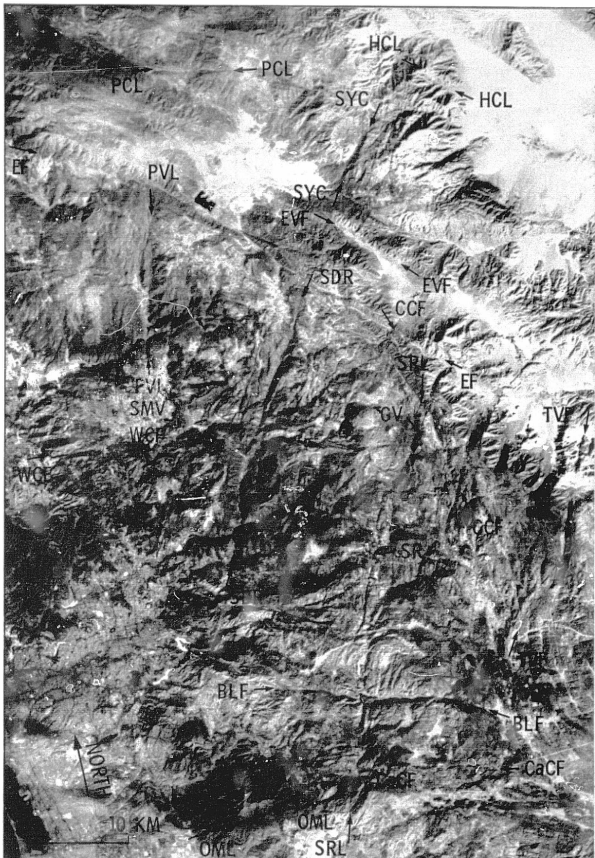
Fig. 4 - Major faults and linears, Peninsular Ranges, southwestern California. Portion of Landsat image 1106-17504. Abbreviations: BLF: Barrett Lake fault; CCF: Chariot Canyon fault; CaCF: Canyon City fault; EF: Elsinore fault; EVF: Earthquake Valley fault; HCL: Henderson Canyon linear; GV: Green Valley; OML: Otay Mountain linear; PCL: Previt Canyon linear; PVL: Pamo Valley linear; SDR: San Diego River fault zone; SMV: Santa Maria Valley; SR: Sweetwater River; SRL: Sweetwater River linear; SYC: San Ysidro Creek fault; TVF: Thing Valley fault; WCF: Warren Canyon fault.
