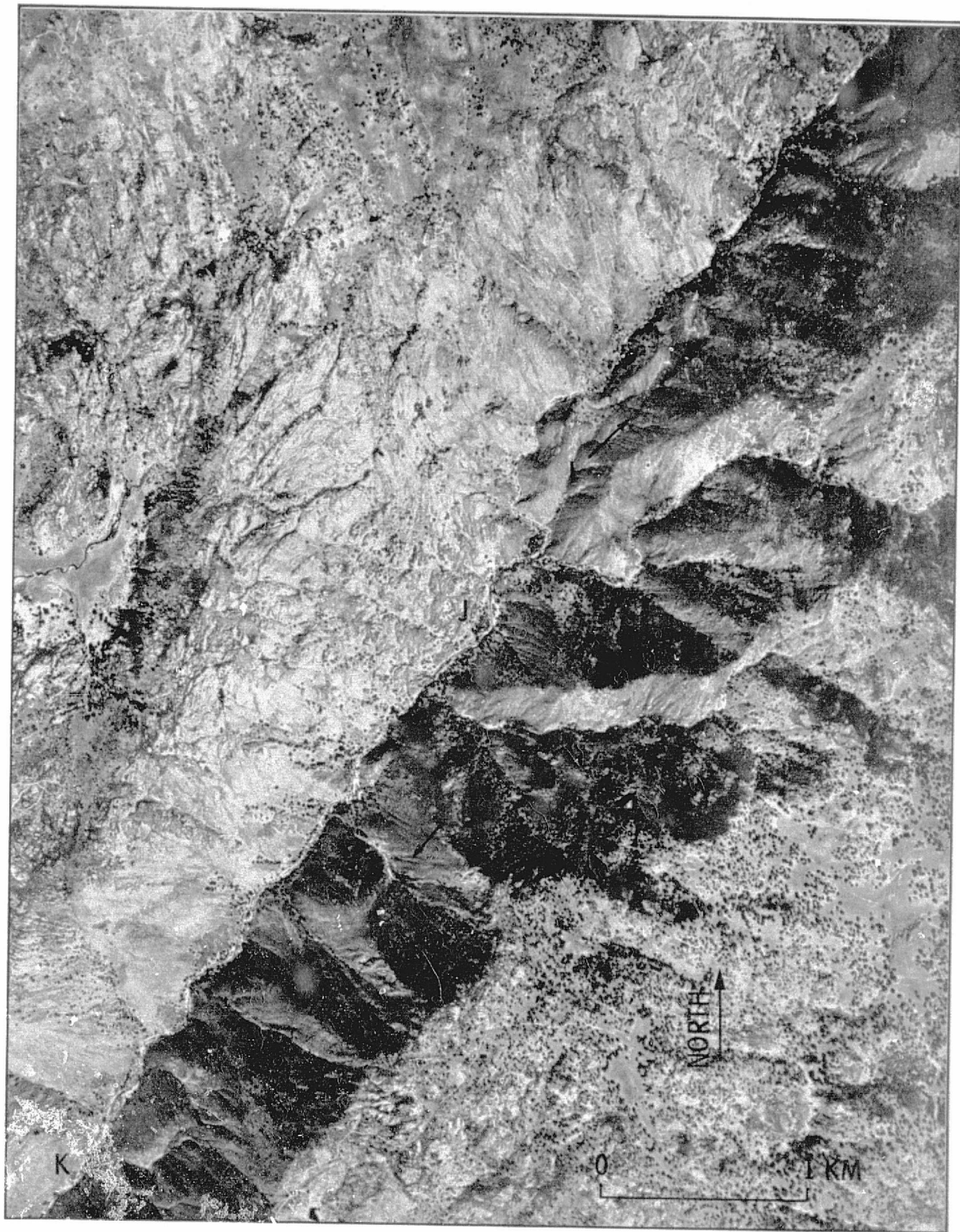
Fig. 20 - Portion of U.S. Department of Agriculture aerial photo number AXN-6M-6, April 2, 1953, showing linears along San Diego River fault zone. Arrows indicate ends of linears and letters keyed to Fig. 13. See Fig. 13 for area covered.
