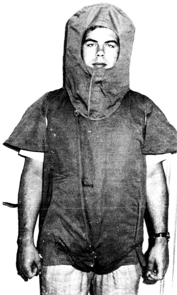
FIGURE 13.—Antinoise suit designed to provide general protection of the organism in intense noise.
