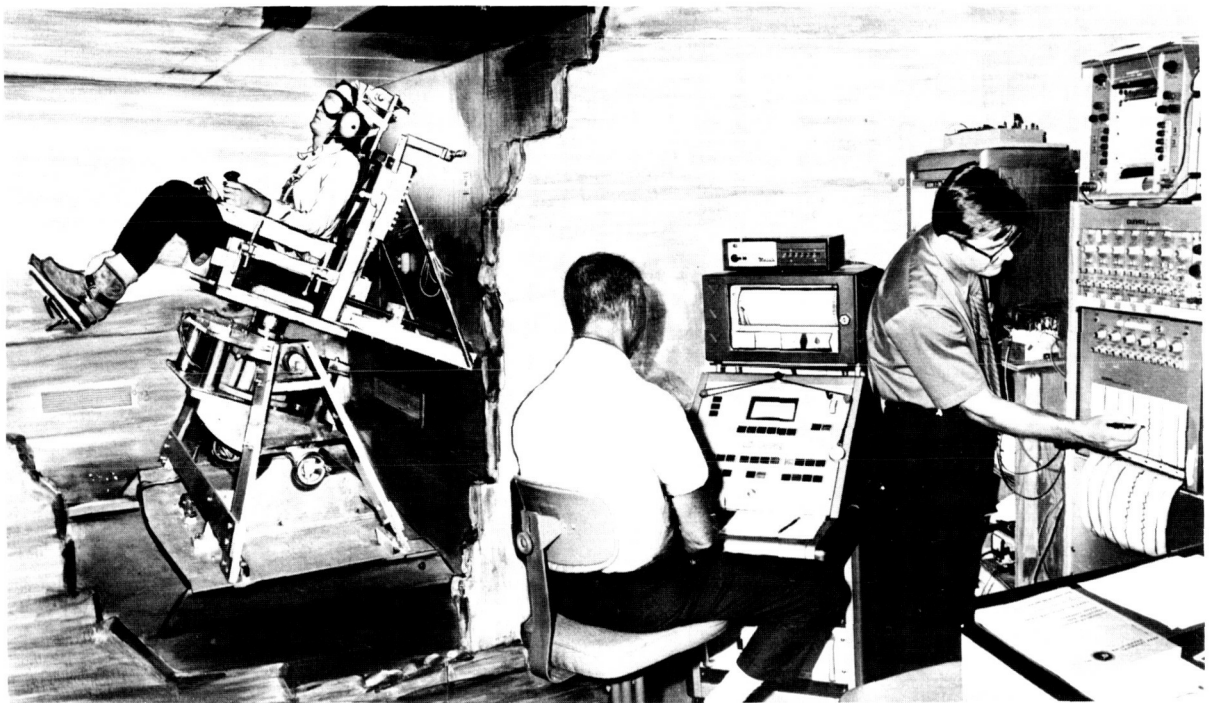
FIGURE 26.—Off-vertical rotating chair device with recording equipment. Chair may be used upright for stimulating semicircular canals and in off-vertical (at constant angular velocity) for stimulating otolith organs. Instrumentation permits fairly complete programming.
