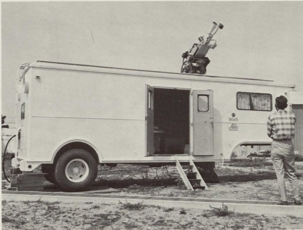
Fig. 3. The Water Vapor Radiometer mounted on its trailer for field testing
