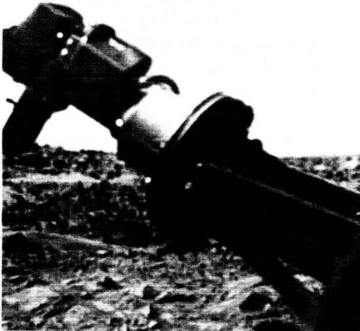
FIGURE 5-2.—The sampler at its correct extension.
