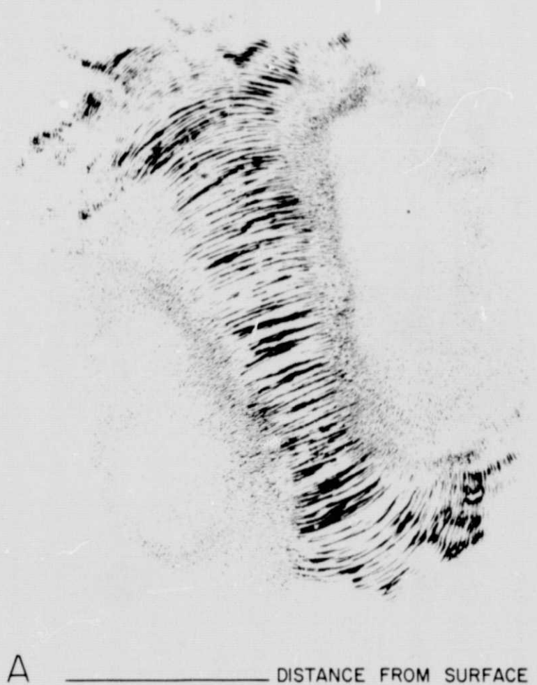
Figure 1. Magnetic field pattern 9 centimeters above the surface of USNM 99484 (the scale bar is 9 cm)
