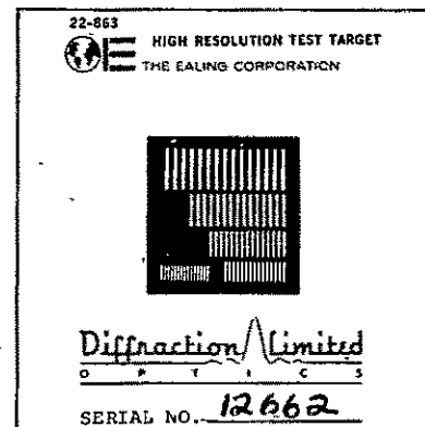
Actual size 6 mm x 16 mm target on 2 inch square plate
