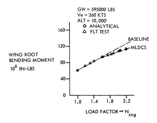
C-5 MLDCS COMPARISON OF ANALYTICAL AND FLIGHT TEST LOADS
