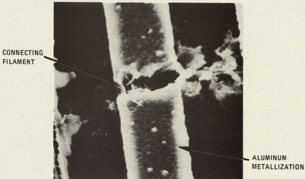
SCRAPE IN "Ø 4 SHIFT" METALLIZATION STRIPE. 1200X
