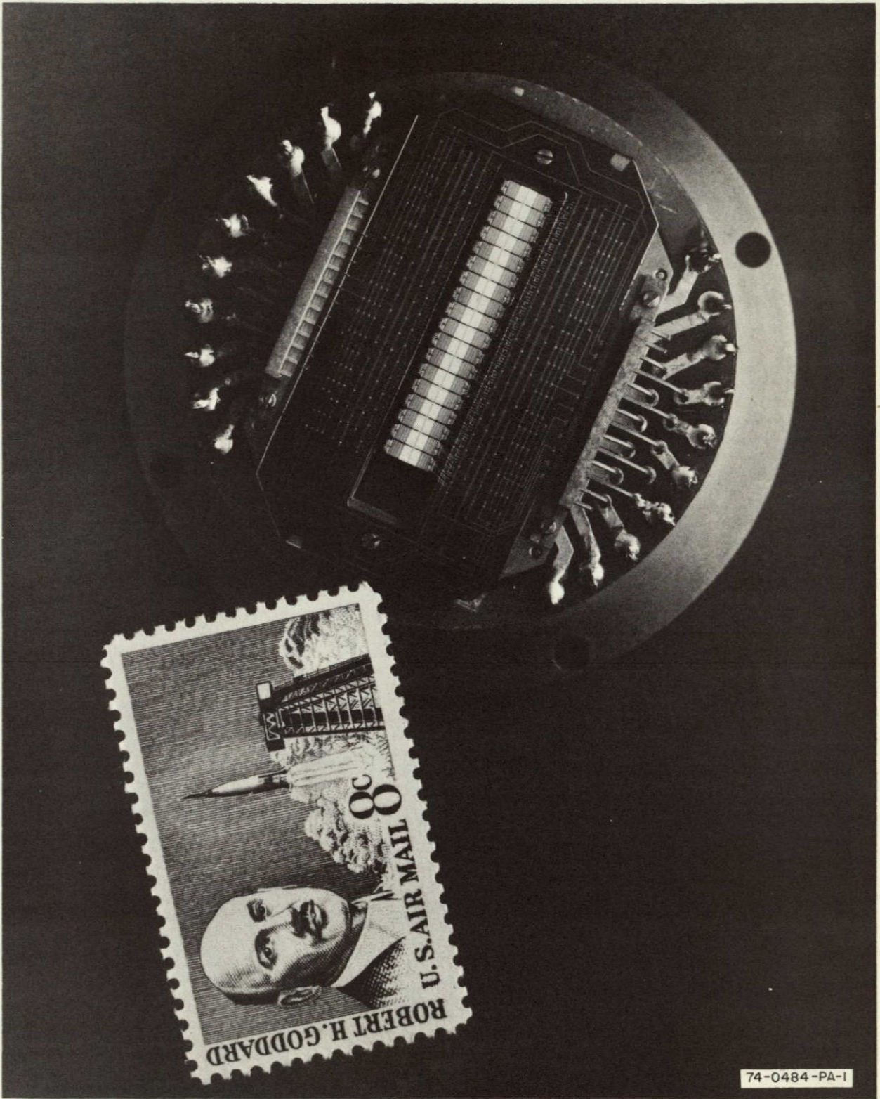
Figure 25. Fully Assembled 1728-Detector Focal Plane Array
