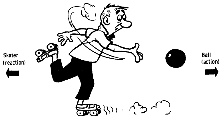
Figure 2-2. - Newton's Third Law of Motion. Reaction - For every acting force there is always an equal and opposite reacting force.
