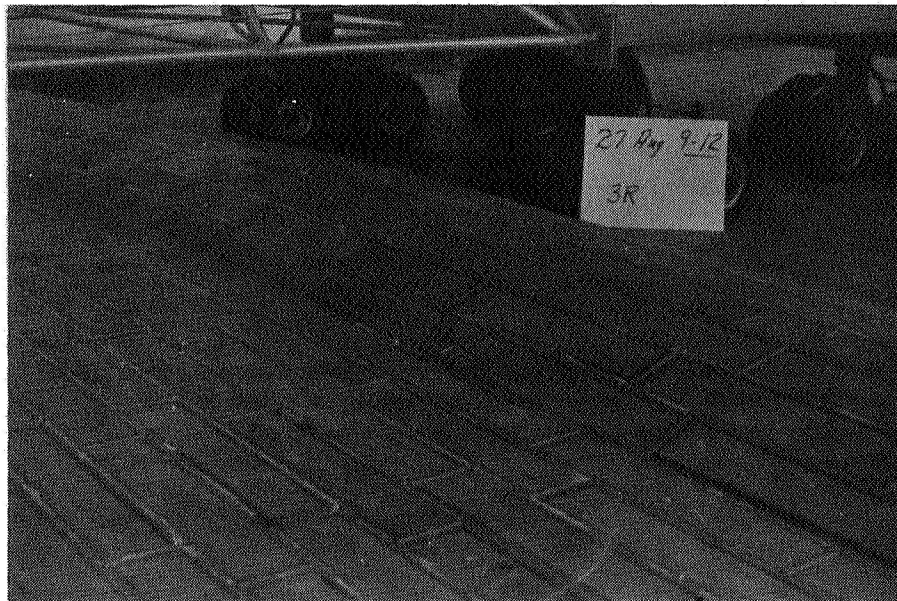
Figure 4.- A typical buckling failure.
