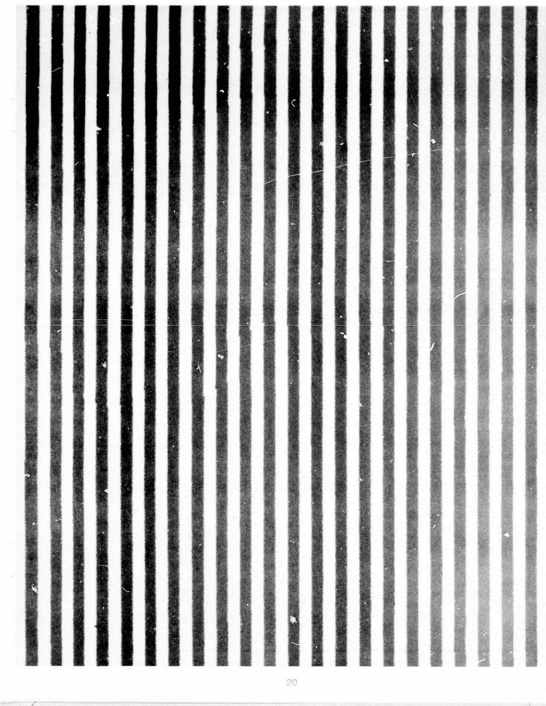
The extent of the shear problem was evaluated by contact photography of a 250 lp/inch Ronchi ruling through the 156mm diameter faceplate. The data were recorded on IIIaJ film at two position angles  $45^{\circ}$  apart. The photographs were enlarged by a factor of ten and examined for shears which appeared as breaks in the ruling. By combining the results from the two position angle plates it was possible to identify all of the shears to a limit of about  $6\mu$  displacement.
