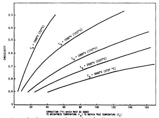
Figure 8. Temperature Corrections for Monochromatic Brightness Pyrometer Employing 65-Micron Wavelength
