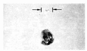
d. 40% CaO Laser Glass—Laser beam attenuated to 33% normal remelted once—approximately 50/50 glass and crystal (note tapering of probe indicating dissolution of silica)
