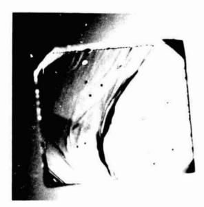
c. Prepared 3/20/75-Striae and Cracks
