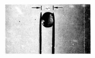
a. 35% CaO Laser Glass--Prepared with laser beam attenuated to 42% normal and remelted once
