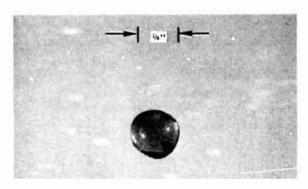
40% CaO Laser Glass--Prepared with laser beam attenuated to 33% normal-remelted twice; note devitrification (two darker zones)
