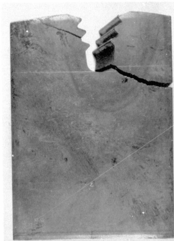
Figure 49 Failed broach block used for root subcomponent LCF test
