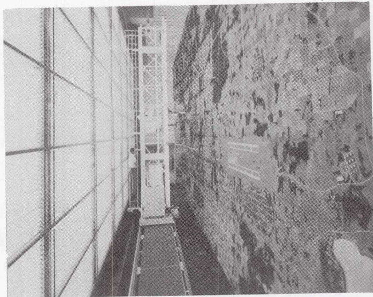
Figure 5.- Photograph of landing scene equipment and airport model.
